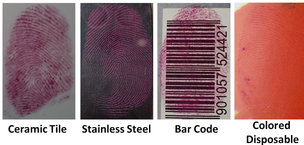
Figure S20b. The photographs of LFPs developed using nano porous silica having 10% loading of PDI 2 (w/w) on different coloured surfaces. The LFPs were visualized in daylight.
