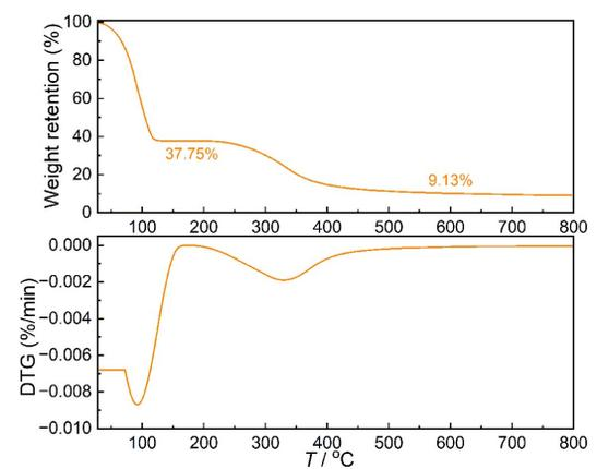
**Figure S5** TG/DTG curves of FK-CS hydrogel.
