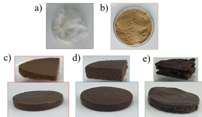
**Figure S12** Specimens of raw material, PFM, the keratin hydrogel and hydrogel composites, (a) duck feathers, (b) PFM, (c) **FK-1** hydrogel, (d) **FK-SP-1** hydrogel, and (e) **FK-CS** hydrogel.
