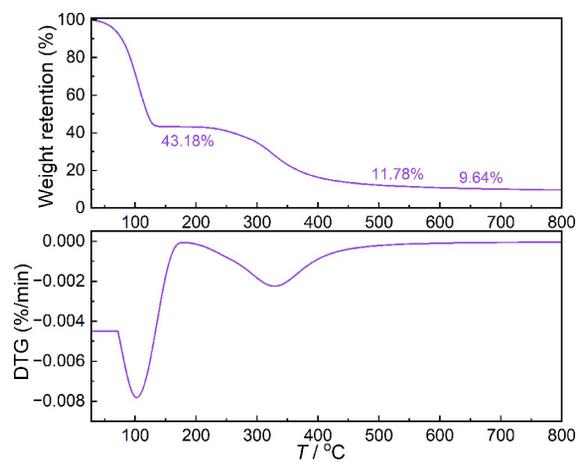
**Figure S6** TG/DTG curves of **FK-Rh B** hydrogel.
