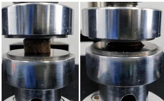
**Figure S10** The diagram of compression process of **FK-1** hydrogel using a mechanical testing machine
