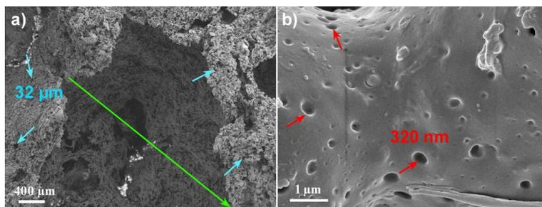
**Figure S8** SEM images of (a) the FK-SP-2 aerogel ( $\times 25$ ), and (b) the FK-SP-2 aerogel ( $\times 15,000$ ). The primary hole structure, the secondary hole structure, and the tertiary pore structure are colored in green, blue, and red, respectively. The primary hole structure of FK-SP-2 sample is very large, and it is difficult to show the whole hole from SEM. Pore sizes of the secondary and tertiary hole structures ranged from 10 to 100  $\mu\text{m}$  and 100 to 500 nm, respectively.
