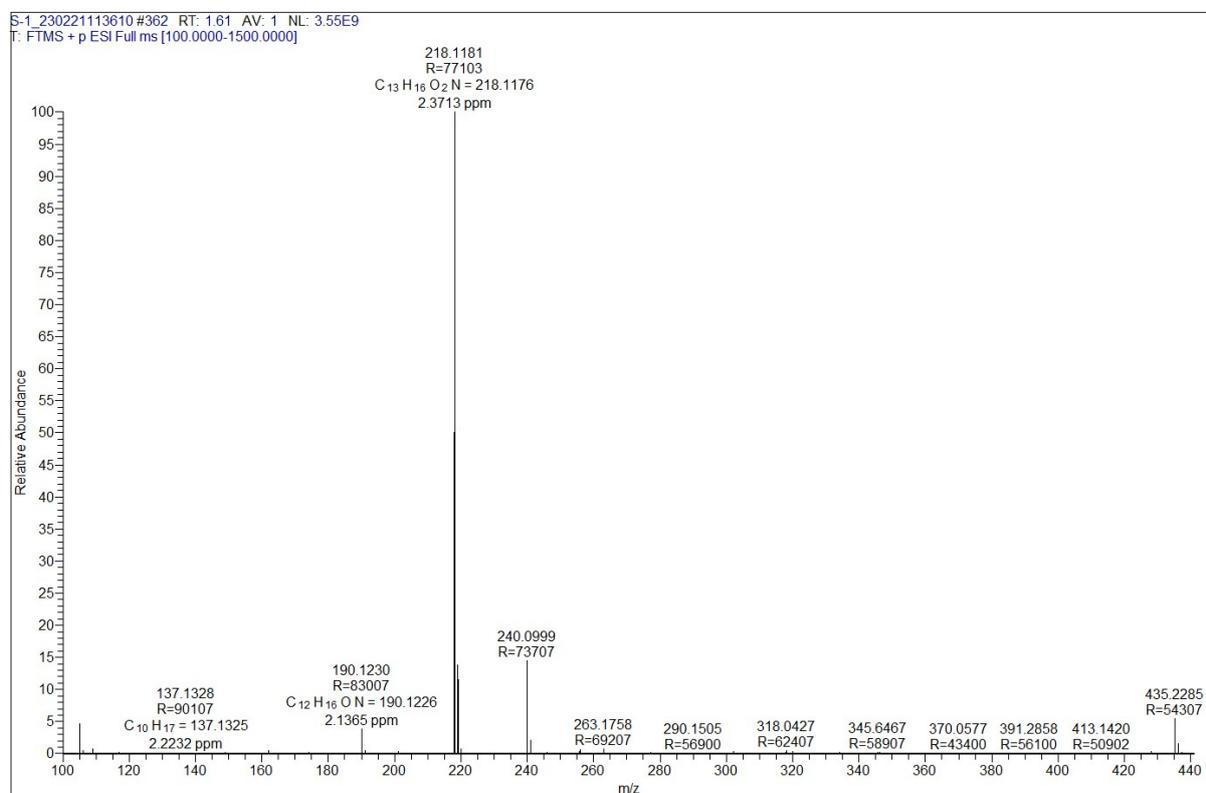
**Fig 4: HRMS of 1-phenyl-2-(piperidin-1-yl)ethane-1,2-dione (3a)**
