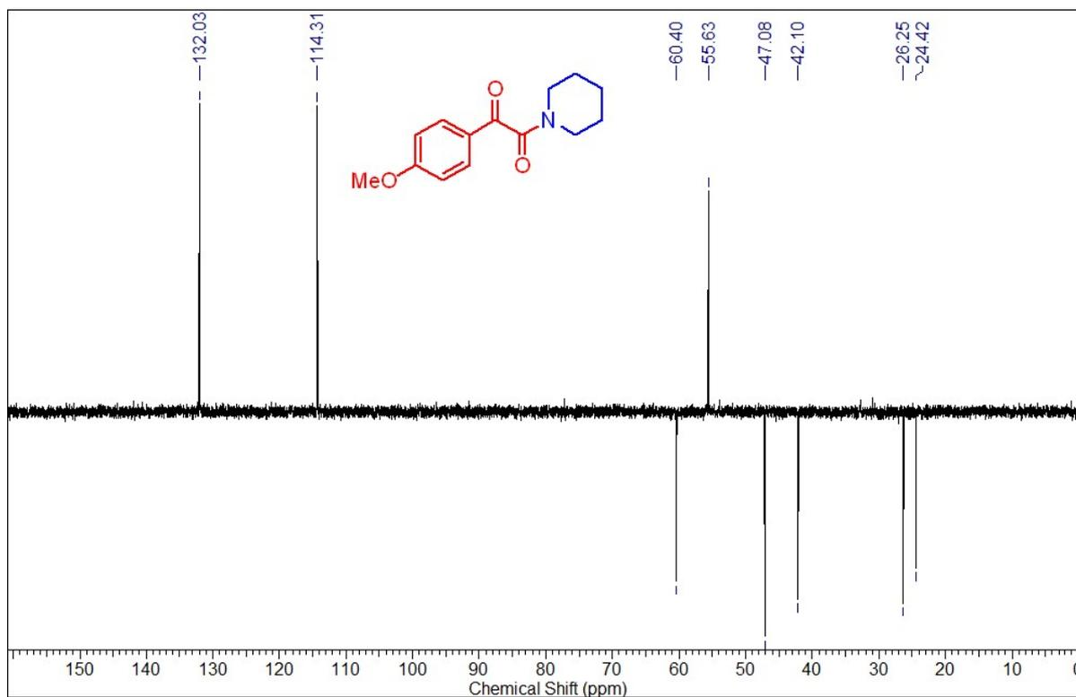
**Fig 55: DEPT (100 MHz, CDCl<sub>3</sub>) of 1-(4-methoxyphenyl)-2-(piperidin-1-yl) ethane 1,2-dione (3n)**
