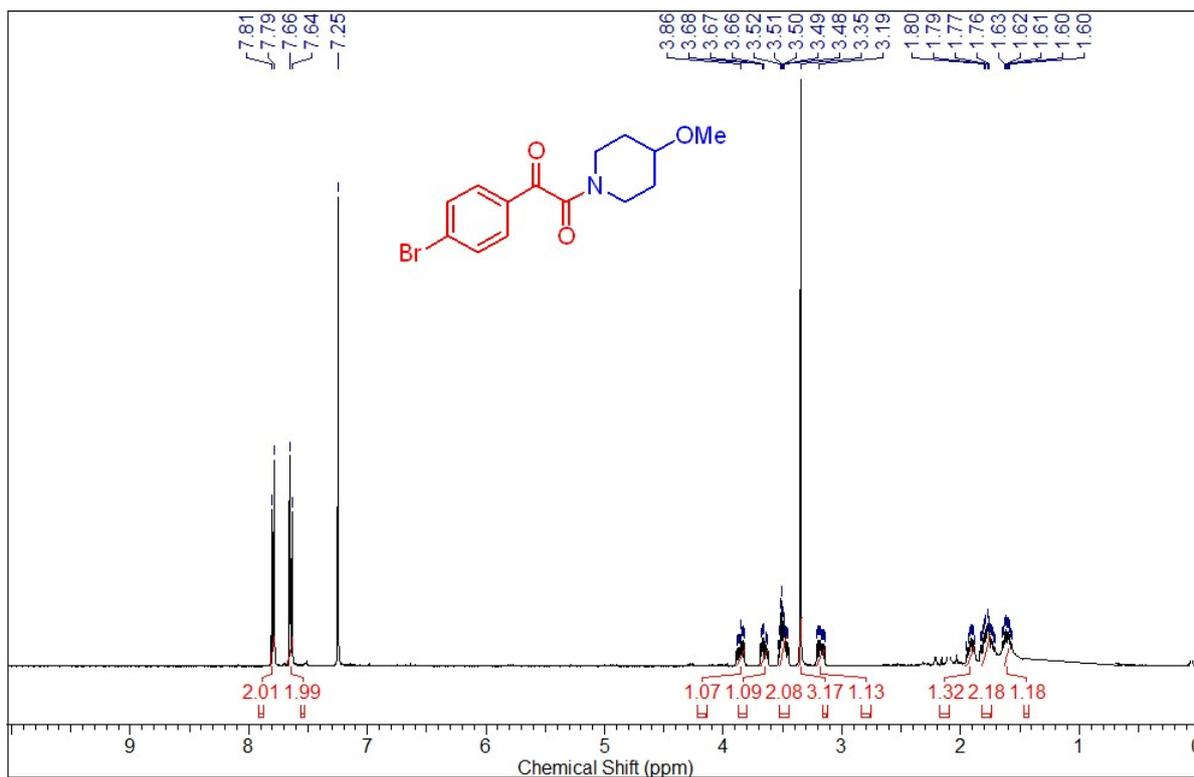
**Fig 49:** <sup>1</sup>H NMR (400 MHz, CDCl<sub>3</sub>) of 1-(4-bromophenyl)-2-(4-methoxypiperidine-1-yl)ethane-1,2-dione (3m)
