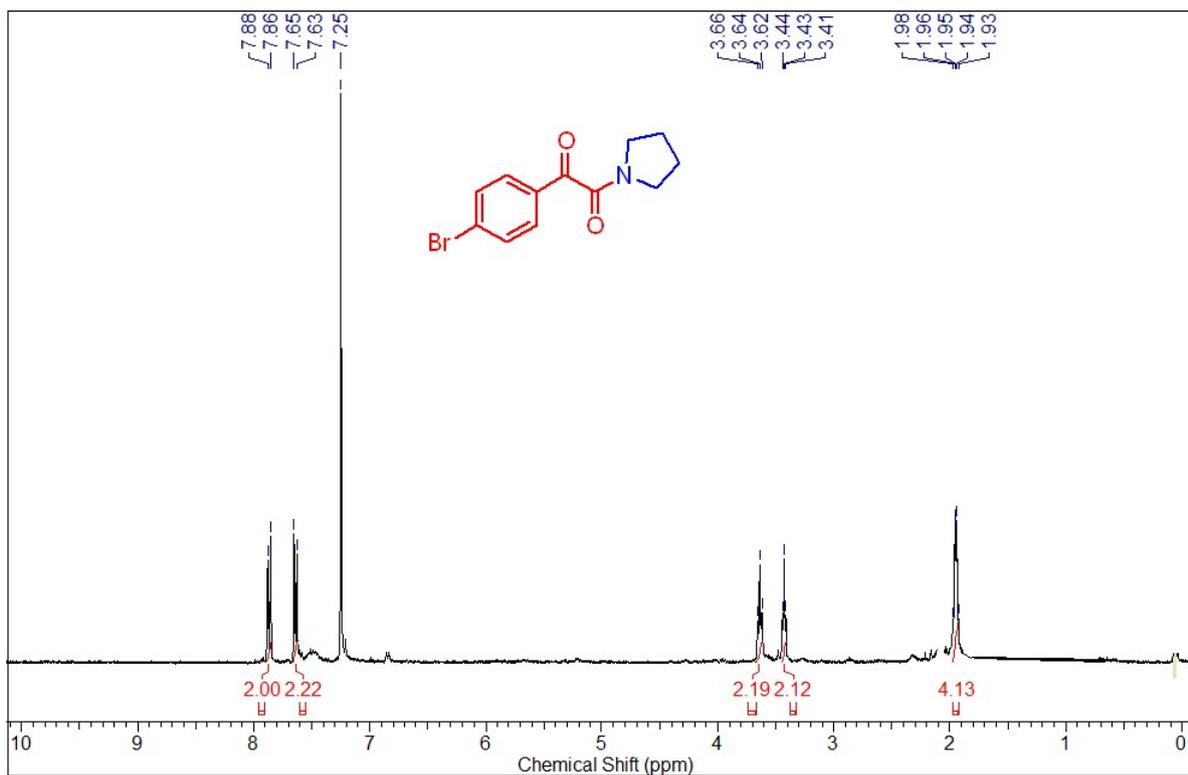
**Fig 37:**  $^1\text{H}$  NMR (400 MHz,  $\text{CDCl}_3$ ) of 1-(4-bromophenyl)-2-(pyrrolidin-1-yl)ethane-1,2-dione(3j)
