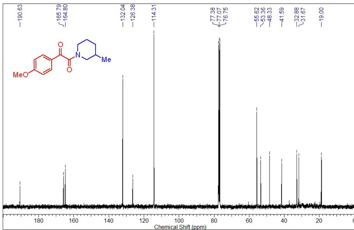
**Fig 66:** <sup>13</sup>C (100 MHz, CDCl<sub>3</sub>) of 1-(4-methoxyphenyl)-2-(3-methylpiperidine-1-yl)ethane-1,2-dione (3q)
