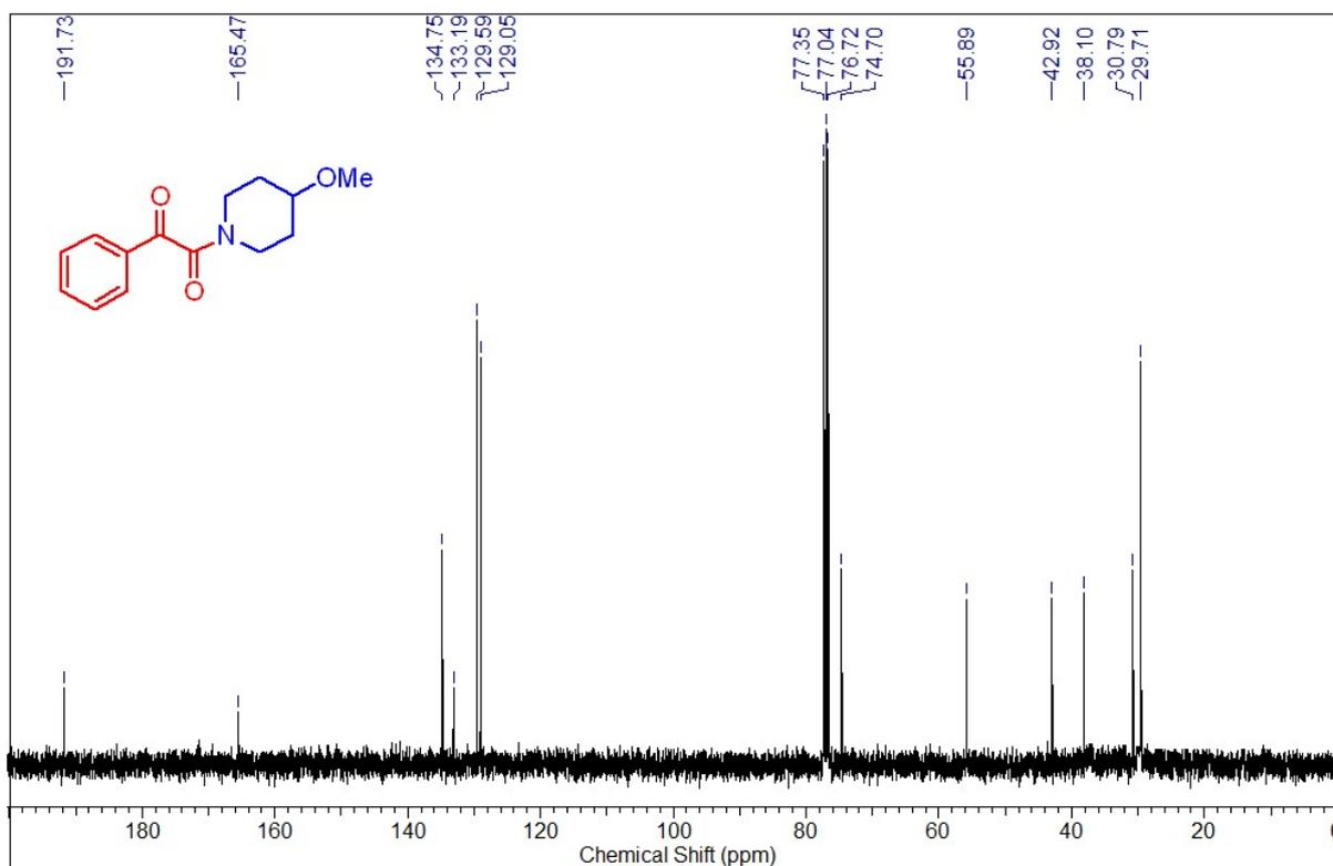
**Fig 26:** <sup>13</sup>C (100 MHz, CDCl<sub>3</sub>) of 1-(4-methoxypiperidine-1-yl)-2-phenylethane-1,2-dione (3g)
