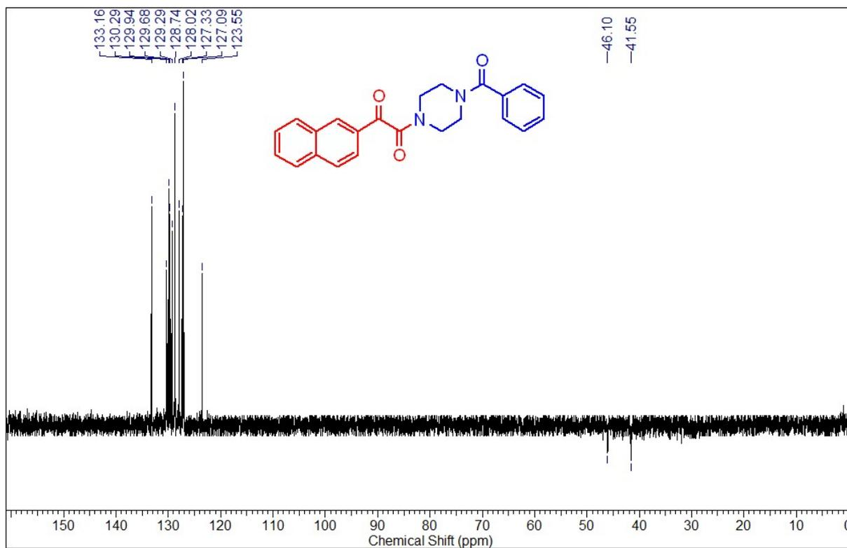
**Fig 79: DEPT (100 MHz, CDCl<sub>3</sub>) of 1-(4-Benzoyl-1-piperazinyl)-2-(2-naphthalenyl)-ethane-1,2-dione (IV)**
