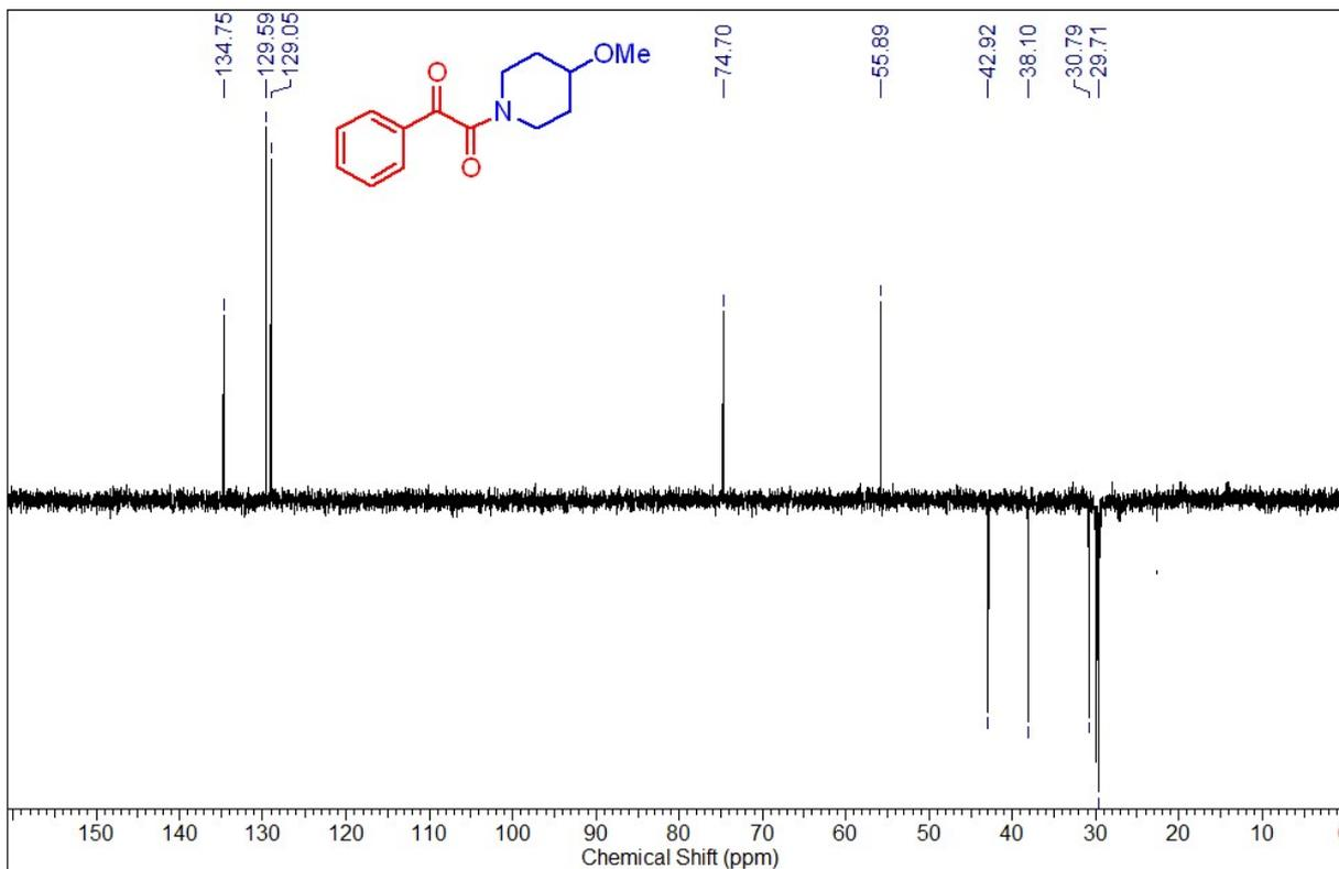
**Fig 27: DEPT (100 MHz, CDCl<sub>3</sub>) of 1-(4-methoxypiperidine-1-yl)-2-phenylethane-1,2-dione (3g)**
