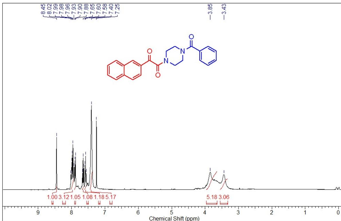
**Fig 77:**  $^1\text{H}$  NMR (400 MHz,  $\text{CDCl}_3$ ) of 1-(4-Benzoyl-1-piperazinyl)-2-(2-naphthalenyl)ethane-1,2-dione (IV)
