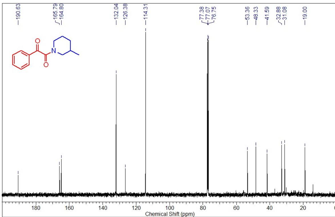
Fig 18:  $^{13}\text{C}$  (100 MHz,  $\text{CDCl}_3$ ) of 1-(3-methylpiperidine-1-yl)-2-phenylethane-1,2-dione (3e)
