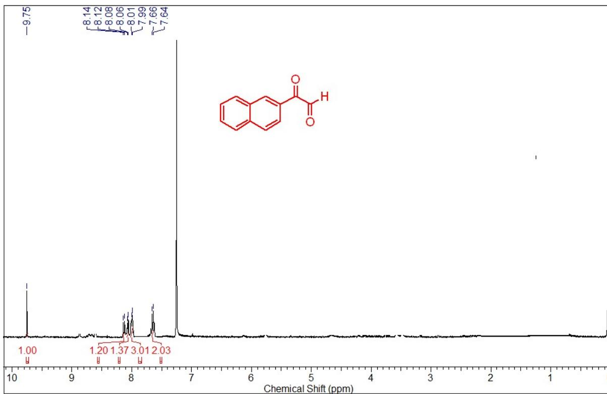
Fig 69:  $^1\text{H}$  NMR (400 MHz,  $\text{CDCl}_3$ ) of 2-naphthalen-2-yl-2-oxoacetaldehyde (6b)
