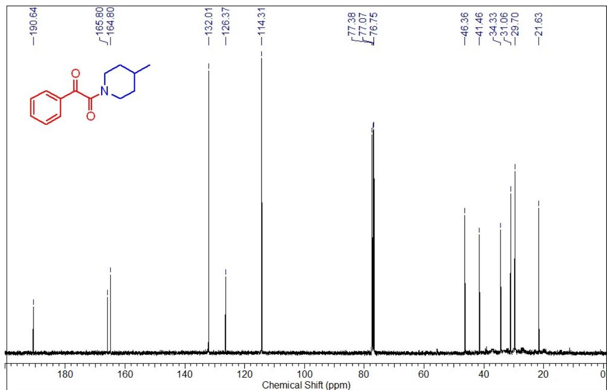
**Fig 14:** <sup>13</sup>C (100 MHz, CDCl<sub>3</sub>) of 1-(4-methylpiperidine-1-yl)-2-phenylethane-1,2-dione (3d)
