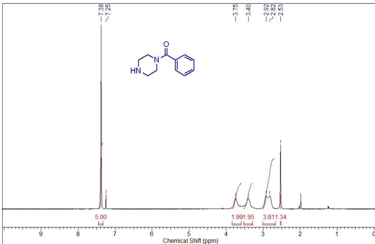
Fig 73:  $^1\text{H}$  NMR (400 MHz,  $\text{CDCl}_3$ ) of 1-benzoyl piperazine
