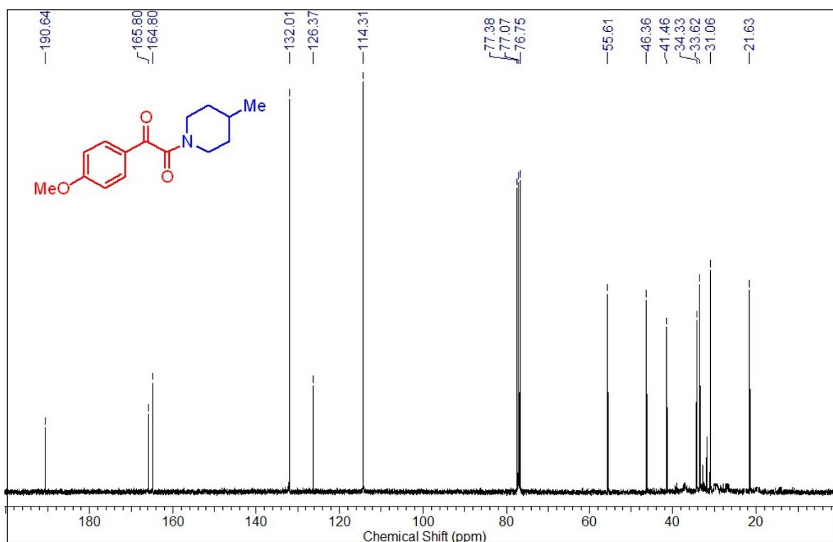
**Fig 62: <sup>13</sup>C (100 MHz, CDCl<sub>3</sub>) of 1-(4-methoxyphenyl)-2-(4-methylpiperidine-1-yl)ethane-1,2-dione (3p)**
