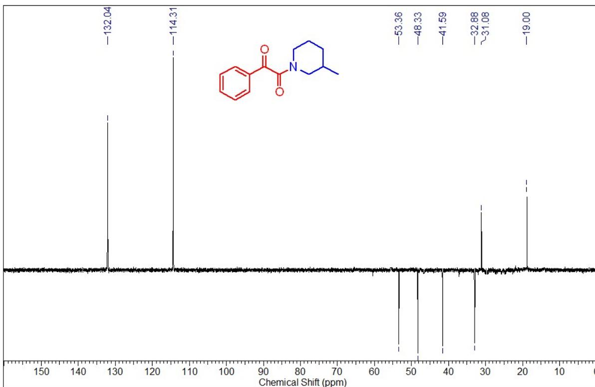
**Fig 19: DEPT (100 MHz, CDCl<sub>3</sub>) of 1-(3-methylpiperidine-1-yl)-2-phenylethane-1,2-dione (3e)**
