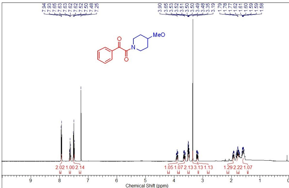
**Fig 25:** <sup>1</sup>H NMR (400 MHz, CDCl<sub>3</sub>) of 1-(4-methoxypiperidine-1-yl)-2-phenylethane-1,2-dione (3g)
