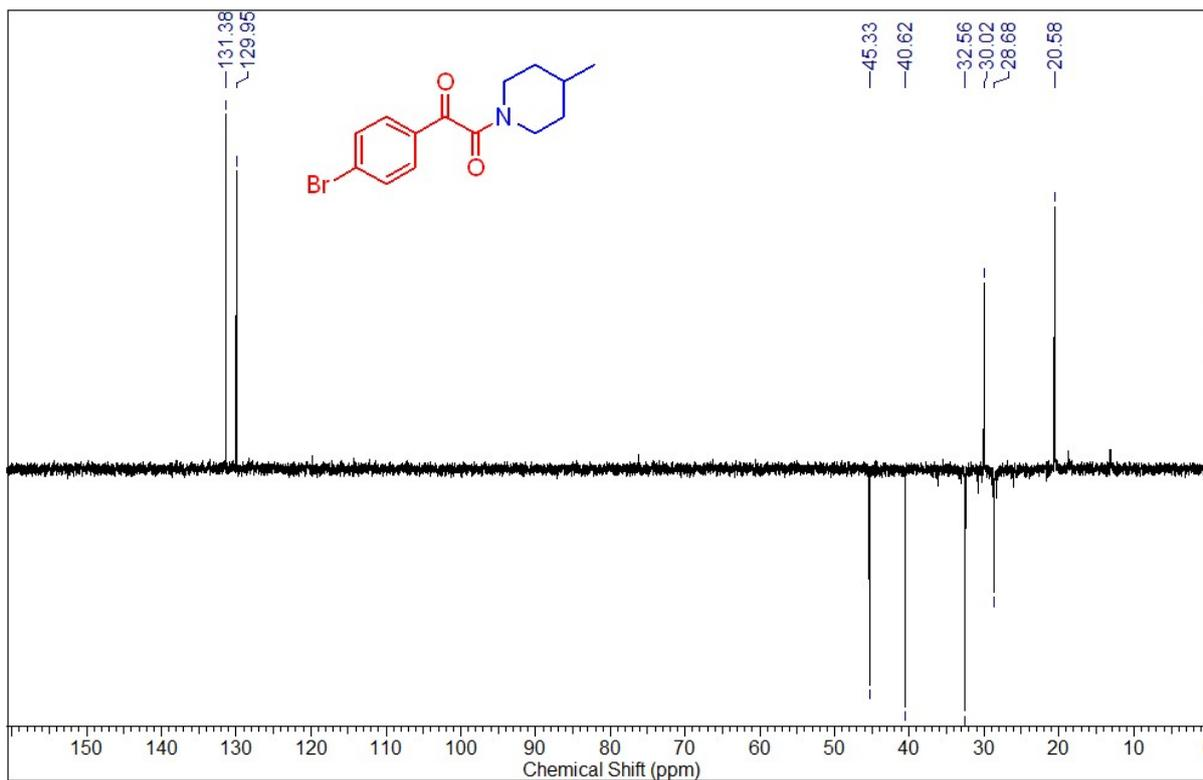
**Fig 43: DEPT (100 MHz, CDCl<sub>3</sub>) of 1-(4-bromophenyl)-2-(4-methylpiperidine-1-yl) ethane-1,2-dione (3k)**
