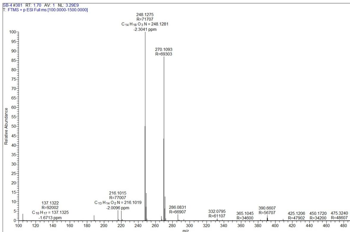
**Fig 28: HRMS of 1-(4-methoxypiperidine-1-yl)-2-phenylethane-1,2-dione (3g)**
