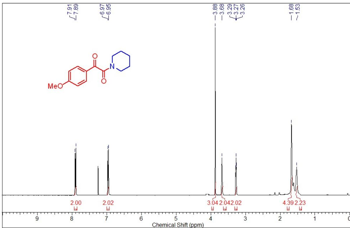
**Fig 53:**  $^1\text{H}$  NMR (400 MHz,  $\text{CDCl}_3$ ) of 1-(4-methoxyphenyl)-2-(piperidin-1-yl) ethane-1,2-dione (3n)
