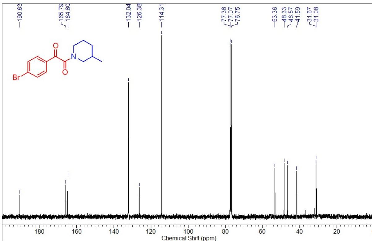
Fig 46: <sup>13</sup>C (100 MHz, CDCl<sub>3</sub>) of 1-(4-bromophenyl)-2-(3-methylpiperidine-1-yl)ethane-1,2-dione (3l)
