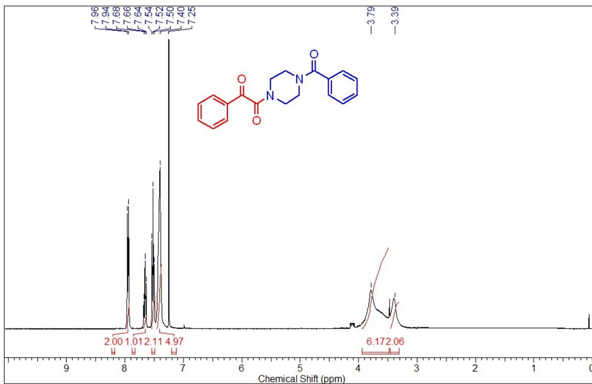
**Fig 29: <sup>1</sup>H NMR (400 MHz, CDCl<sub>3</sub>) of 1-( 4-Benzoyl-1-piperazinyl)-2-phenylethane-1,2-dione (3h)**
