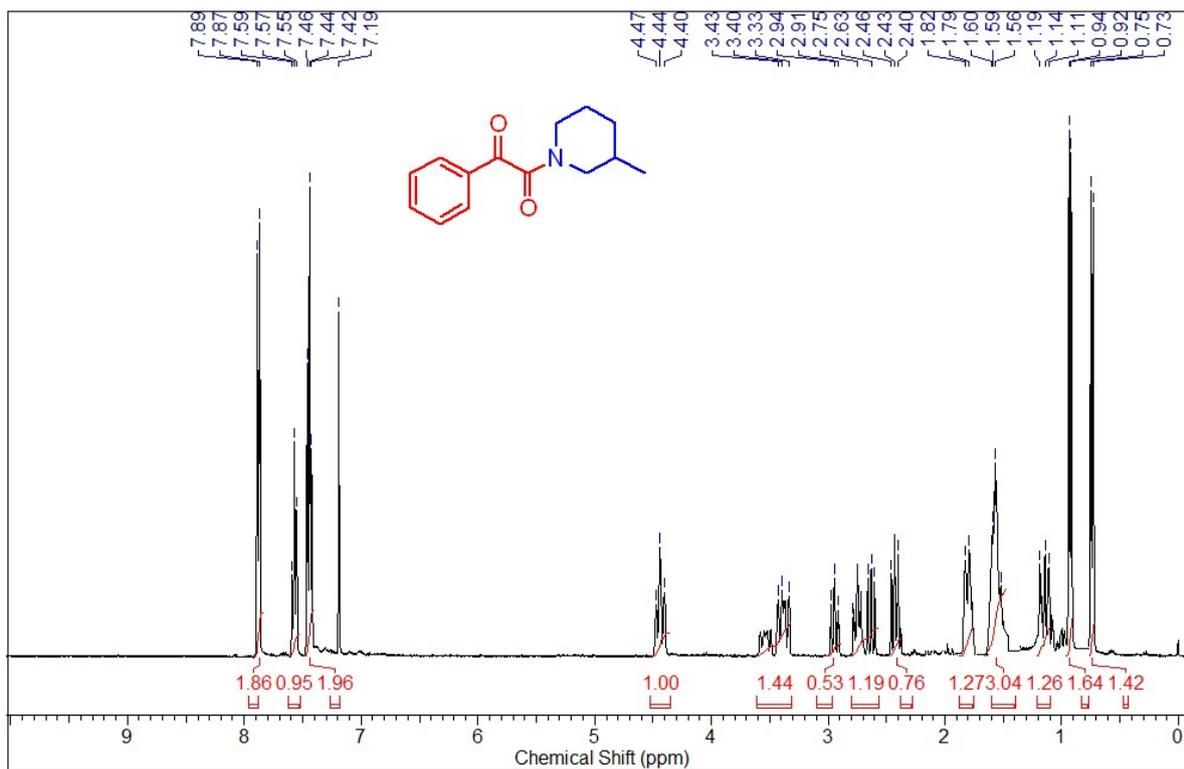
Fig 17:  $^1\text{H}$  NMR (400 MHz,  $\text{CDCl}_3$ ) of 1-(3-methylpiperidine-1-yl)-2-phenylethane-1,2-dione (3e)
