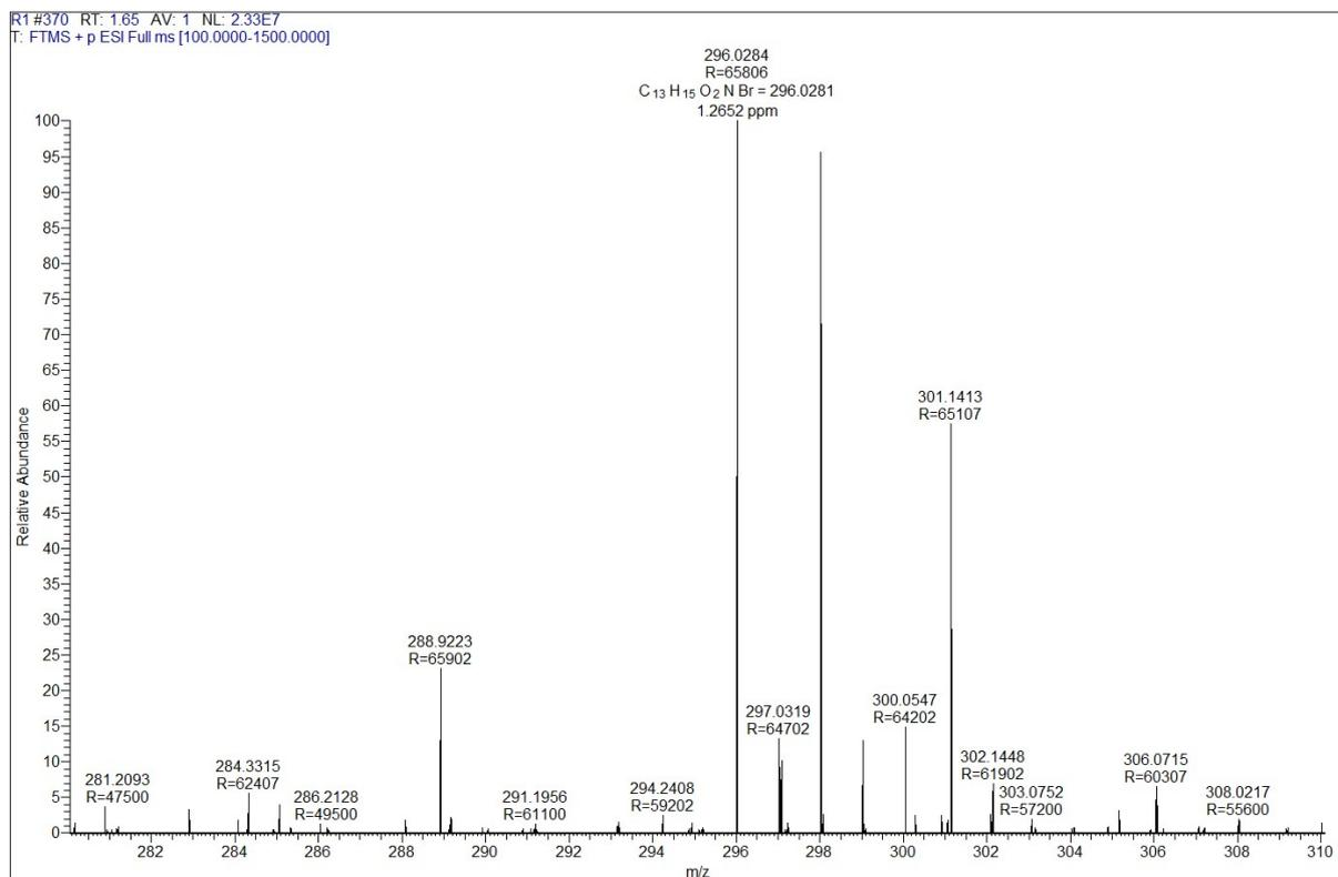
**Fig 24: HRMS of 1-(4-bromopiperidine-1-yl)-2-phenylethane-1,2-dione (3f)**
