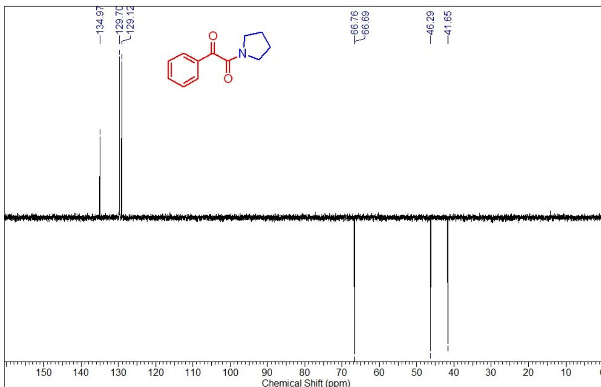
Fig 11: DEPT (100 MHz,  $\text{CDCl}_3$ ) of 1-Phenyl-2-(pyrrolidin-1-yl)ethane-1,2-dione (3c)
