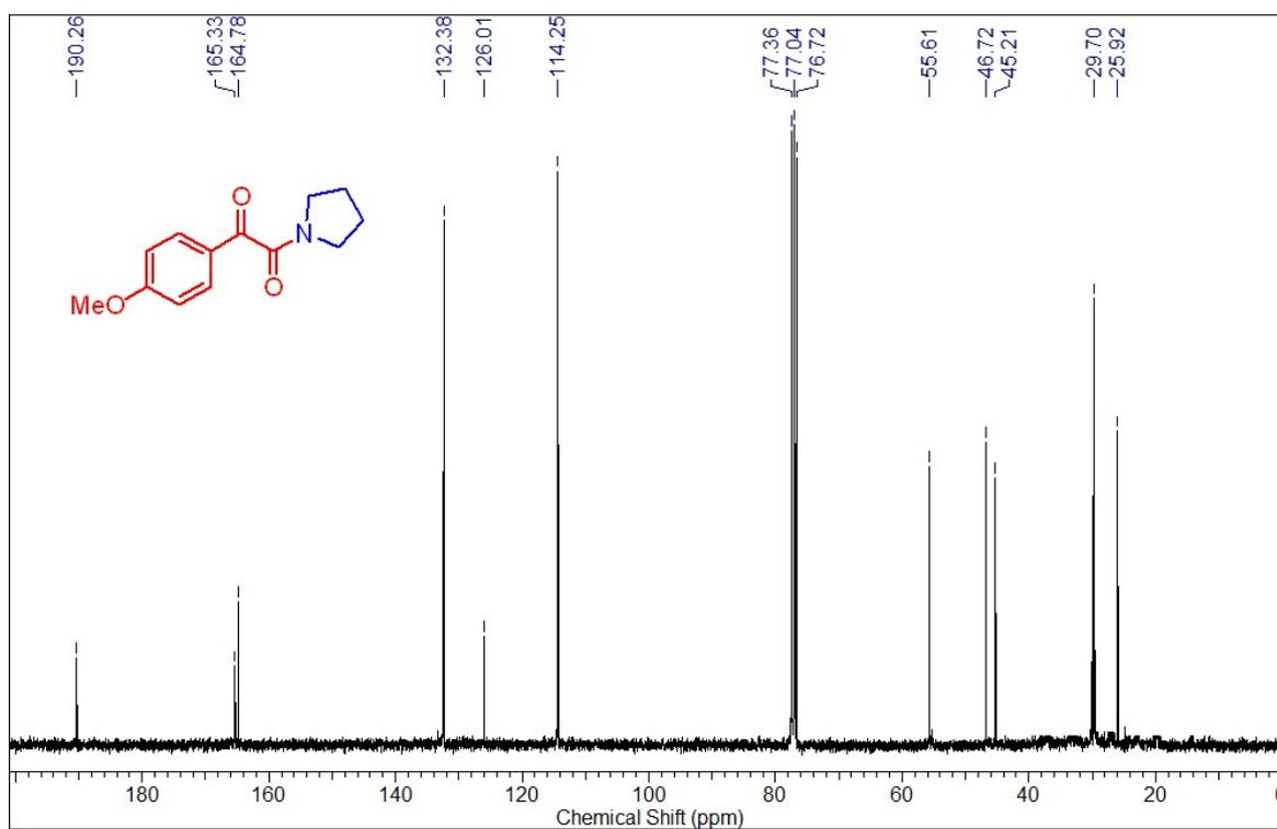
**Fig 58:** <sup>13</sup>C (100 MHz, CDCl<sub>3</sub>) of 1-(4-methoxyphenyl)-2-(pyrrolidin-1-yl) ethane-1,2-dione (3o)
