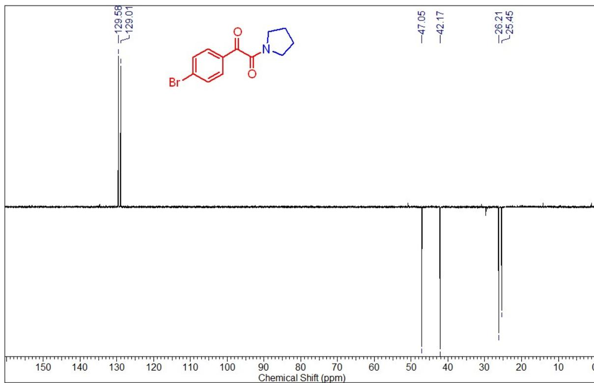
**Fig 39: DEPT (100 MHz, CDCl<sub>3</sub>) of 1-(4-bromophenyl)-2-(pyrrolidin-1-yl)ethane-1,2-dione (3j)**
