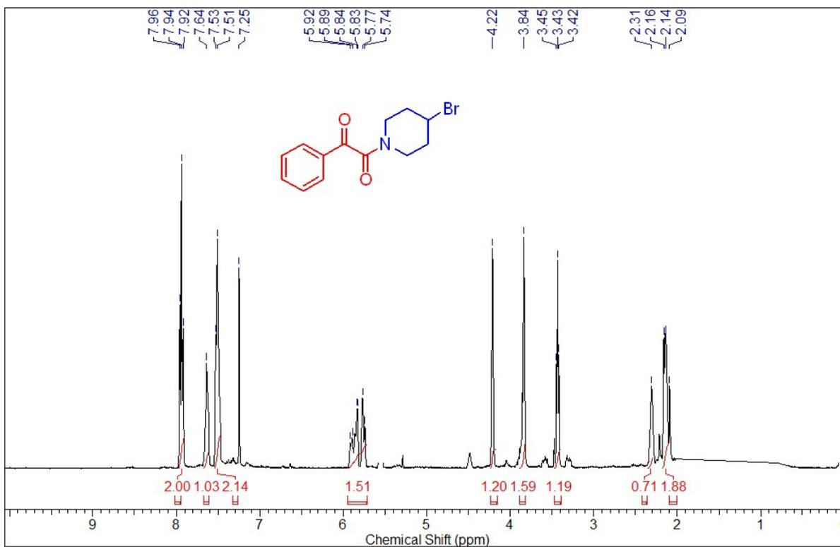
**Fig 21:  $^1\text{H}$  NMR (400 MHz,  $\text{CDCl}_3$ ) of 1-(4-bromopiperidine-1-yl)-2-phenylethane-1,2-dione(3f)**
