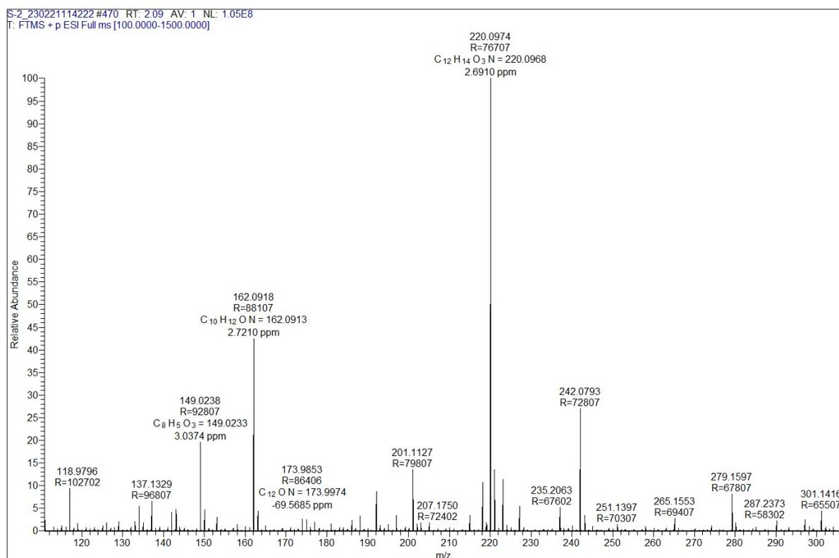
**Fig 8: HRMS of 1-morpholino-2-phenylethane-1,2-dione (3b)**
