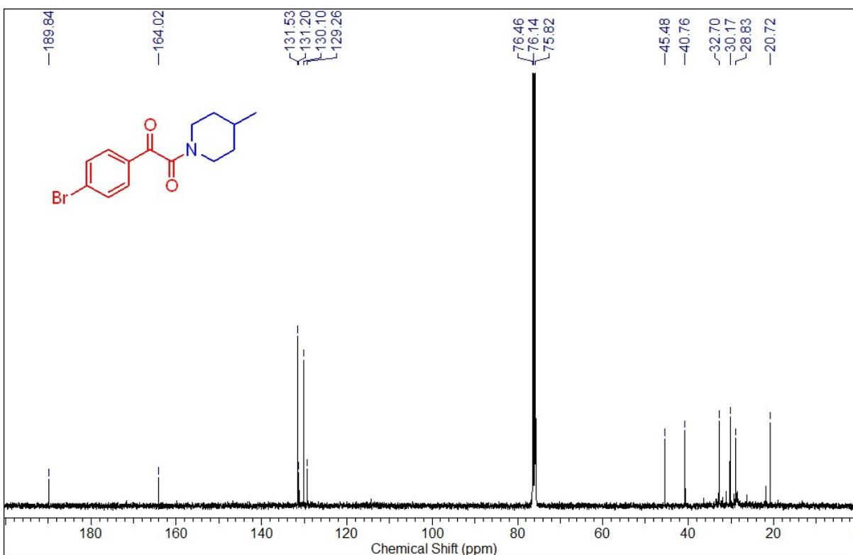
**Fig 42: <sup>13</sup>C (100 MHz, CDCl<sub>3</sub>) of 1-(4-bromophenyl)-2-(4-methylpiperidine-1-yl) ethane-1,2-dione (3k)**
