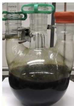
Color of solution after two hours stirring at 160°C
