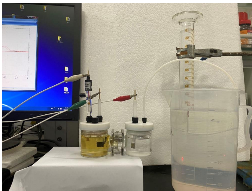
Fig. S25 Diagram of hydrogen collection device in the cathode.
