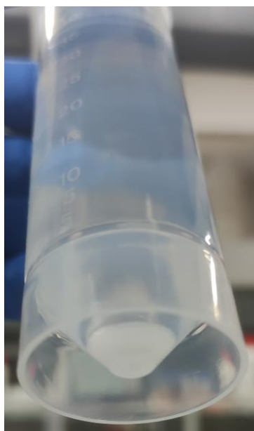
Fig. S17 Diagram of solid products precipitated by sufficient acidification after electrooxidation of HMF.
