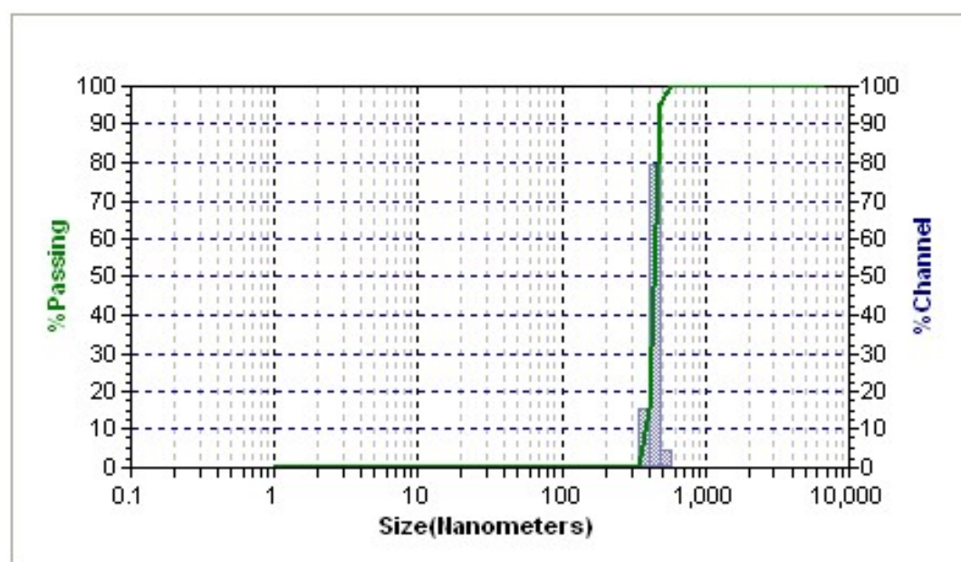
Figure S7. DLS histogram of the nano – aggregates of host (NH-1) upon binding with the bisulphate anions.
