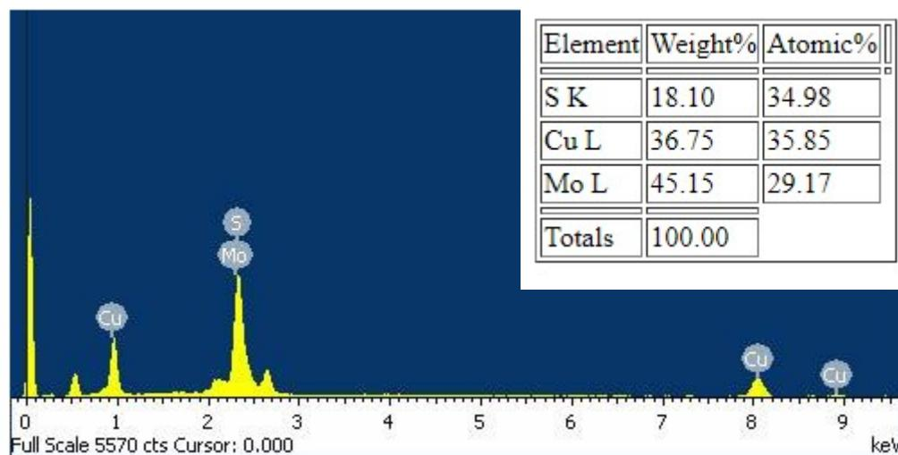
Figure S2 EDX spectrum of MoS<sub>2</sub>/Cu nanozyme (inset: elemental composition)
