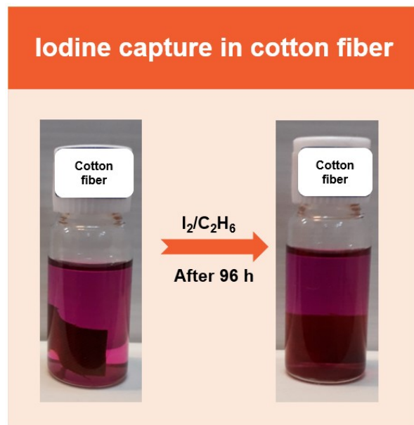
Fig. S7. Color change photograph of cotton fibers which were soaked in I_2 cyclohexane solution (3 mL, 0.0025 M).
