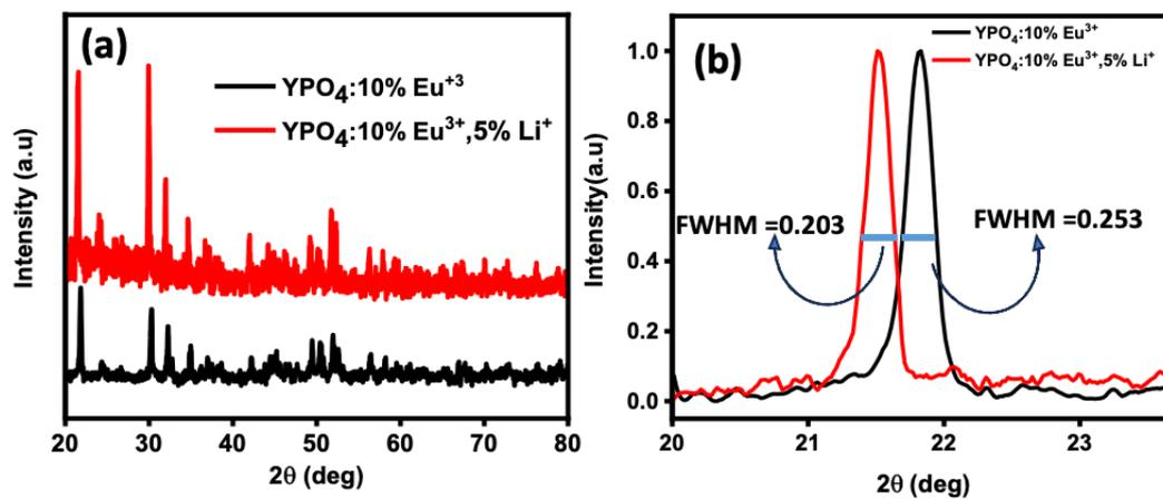
Fig. SI7 (a) pXRD spectra of YPO<sub>4</sub>:10% Eu<sup>3+</sup> and YPO<sub>4</sub>:10% Eu<sup>3+</sup>, 5% Li<sup>+</sup> (b) Zoom out of (a), decreased in  $2\theta$  and sharper peak is evident from the decreased in full width half maxima (FWHM)
