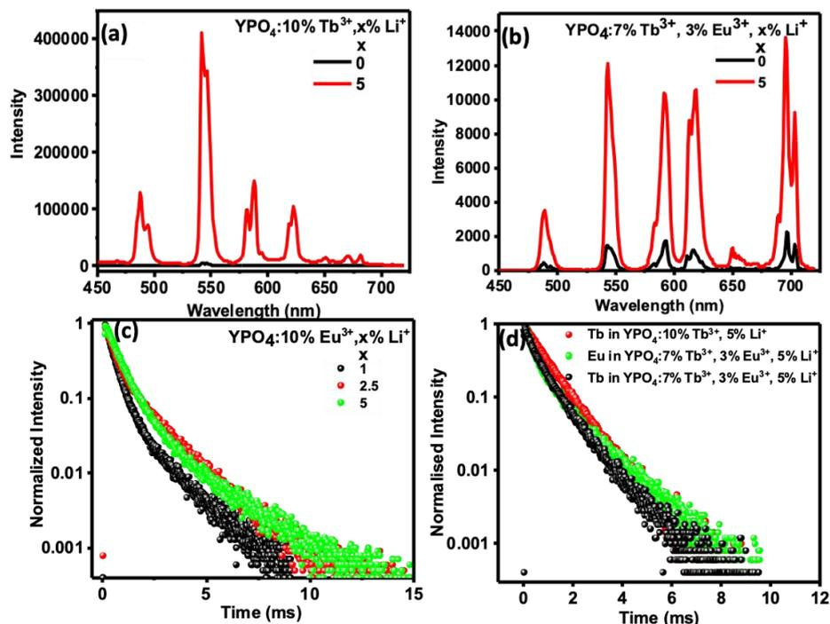
Fig. SI8 (a) Emission spectra of  $\text{YPO}_4:10\% \text{Tb}^{3+}$ ,  $0\% \text{Li}^+$  and  $\text{YPO}_4:10\% \text{Tb}^{3+}$ ,  $5\% \text{Li}^+$  (b)  $\text{YPO}_4:7\% \text{Tb}^{3+}$ ,  $3\% \text{Eu}^{3+}$ ,  $0\% \text{Li}^+$  and  $\text{YPO}_4:7\% \text{Tb}^{3+}$ ,  $3\% \text{Eu}^{3+}$ ,  $5\% \text{Li}^+$  (c) Decay Plot of  $\text{YPO}_4:10\% \text{Eu}^{3+}$ ,  $\text{Li}^+$ , at different  $\text{Li}^+$  % (d) Decay plot of Fig. (a-b).
