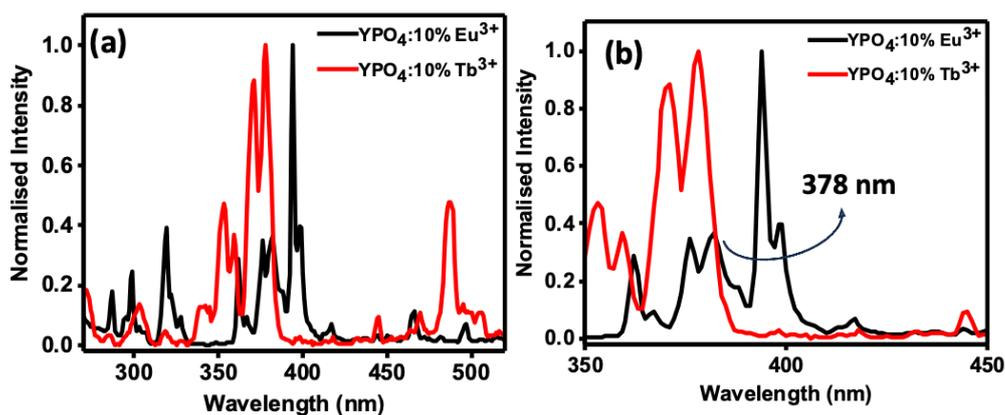
Fig. SI4 (a) Excitation spectra of  $\text{YPO}_4:10\% \text{Eu}^{3+}$  ( $\lambda_{\text{em}} = 700 \text{ nm}$ ) and  $\text{YPO}_4:10\% \text{Tb}^{3+}$  ( $\lambda_{\text{em}} = 545 \text{ nm}$ ) (b) Zoom out image of Fig. a, there is an overlap between  $\text{YPO}_4:10\% \text{Eu}^{3+}$  and  $\text{YPO}_4:10\% \text{Tb}^{3+}$ , there is an overlap between them at 378 nm and it was used as the excitation wavelength for measuring all the emission spectra.
