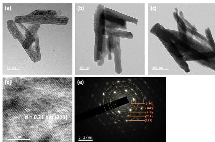
Fig. SI3 (a-c) TEM images of  $\text{YPO}_4:7\% \text{Tb}^{3+}, 3\% \text{Eu}^{3+}$  (d) HRTEM image of  $\text{YPO}_4:7\% \text{Tb}^{3+}, 3\% \text{Eu}^{3+}$  (e) SAED pattern of  $\text{YPO}_4:7\% \text{Tb}^{3+}, 3\% \text{Eu}^{3+}$
