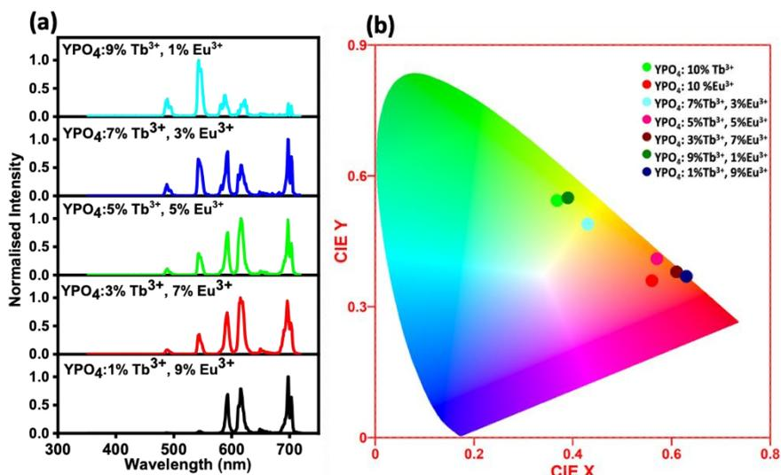
Fig. SI5 (a) Emission Spectra of  $\text{YPO}_4:\text{Tb}^{3+}, \text{Eu}^{3+}$  at different Tb:Eu ratio ( $\lambda_{\text{ex}} = 378 \text{ nm}$ ) (b) CIE plot of  $\text{YPO}_4: \text{Tb}, \text{Eu}$  at different Tb:Eu ratio
