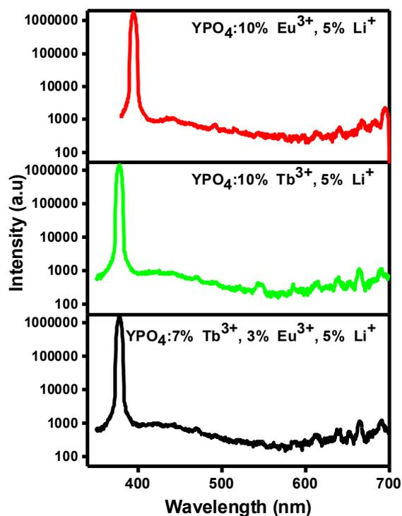
Fig. SI9. Quantum Yield plot of  $\text{Li}^+$  doped  $\text{YPO}_4:\text{Ln}$  nanoparticles using FLS980 Fluorimeter's Integrating Sphere
