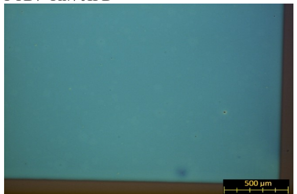
Figure S57. Morphology of PTB7-Th C70 solar cells active layers as observed by microscope with differential interference contrast (5X magnification).
