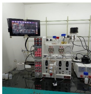
Figure 1. Flow reactor: VAPOURTEC R series, Instrument serial no. P1720, Software: VI.222, pump: VAPOURTEC R2C.
