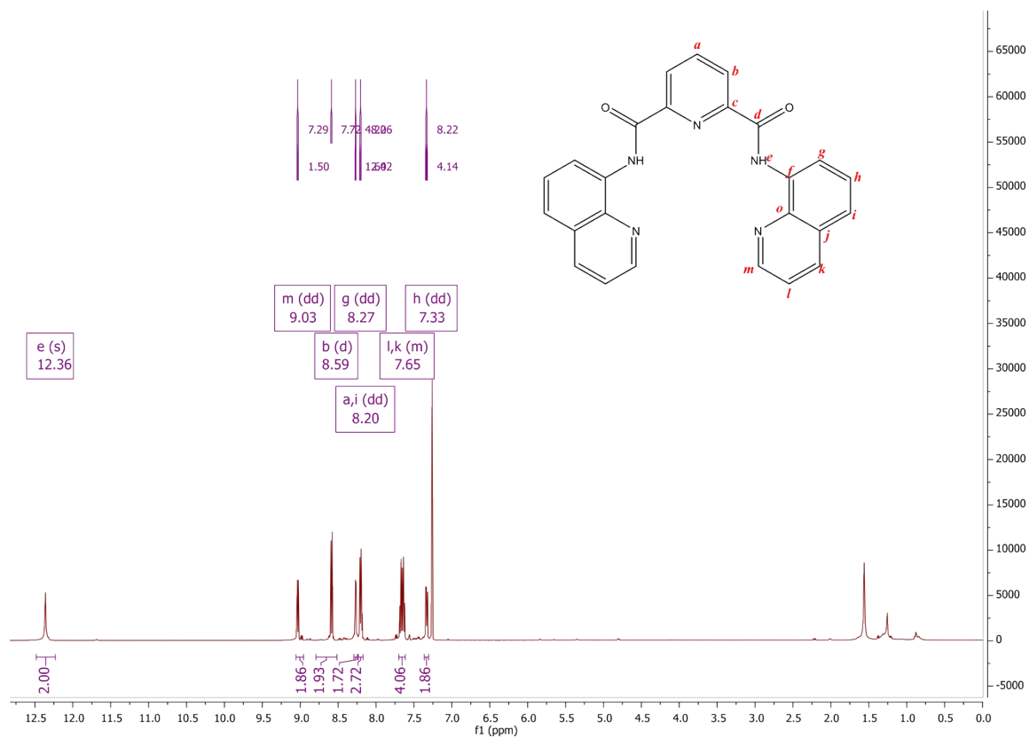
Figure S9. ^1\text{H} (a) and ^{13}\text{C} APT (b) NMR spectra of 1c in DMSO- d_6 .
