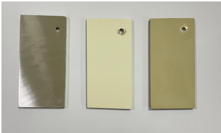
Fig. S1 The image of the sample from left to right is the Mg substrate, before and after reduction under H_2/Ar .
