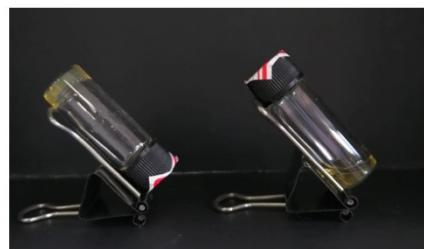
Figure. S7. Molecular structure of Fmoc-GGGG. (B) Gel pictures of Fmoc-GGGG (2%) without (left) or with 2 eq SEB- \beta -CD (right).
