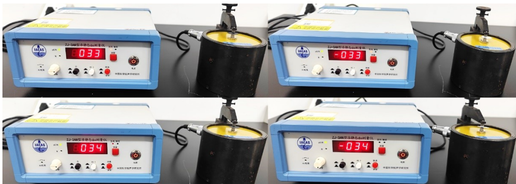
Fig. S5. d_{33} values of the PP/PBTO surface. The front side of PP/PBTO is positively charged, while the reverse side is negatively charged, meaning the electropositivity of PP/PBTO surface.
