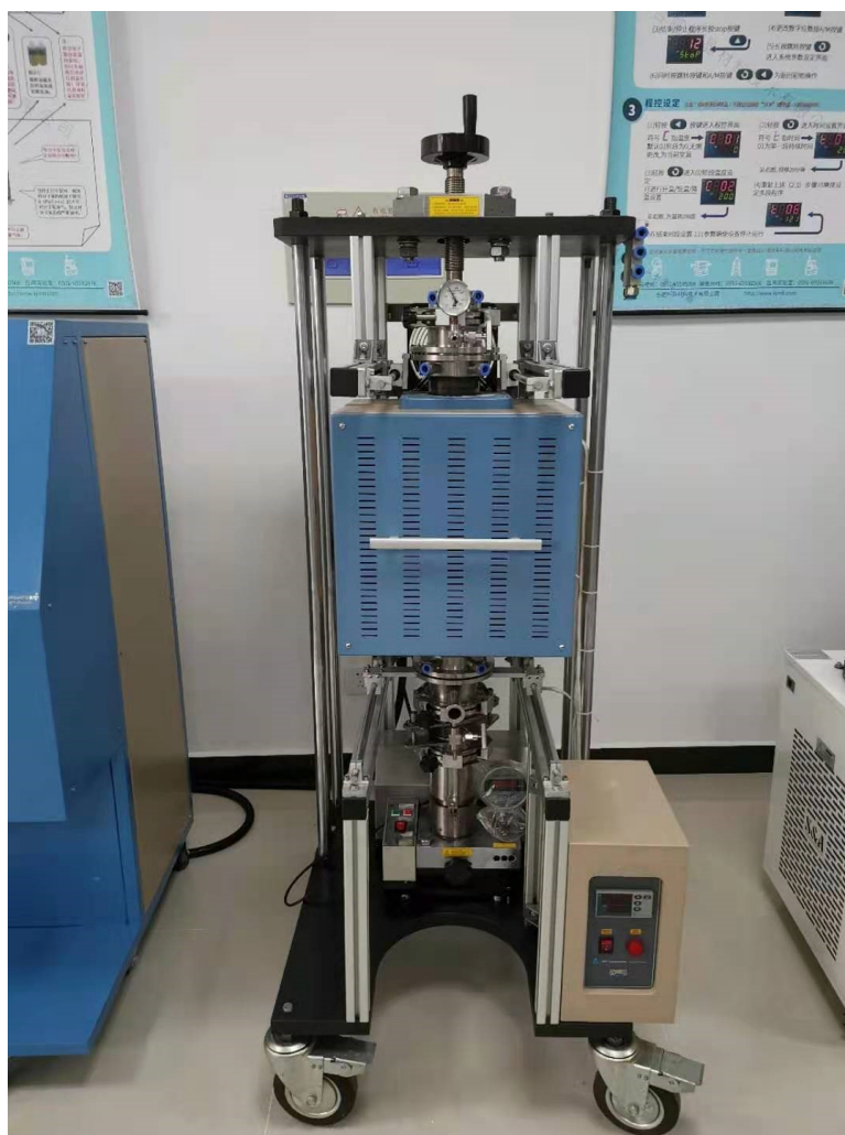
Figure S1. The hot-pressed machined used for fabricating ZIF-62 glass. The model is OTF-1200X-VHP4, more information can be found on the official website of Hefei Kejing Materials Technology Co., Ltd. ( http://www.kjmti.com/product/14182.html ).
