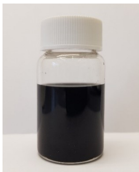
Figure S9. Dispersion of pristine CNHs (1 mg/ml, \text{CHCl}_3 ) four weeks after preparation. This illustrates the stability of the sample.
