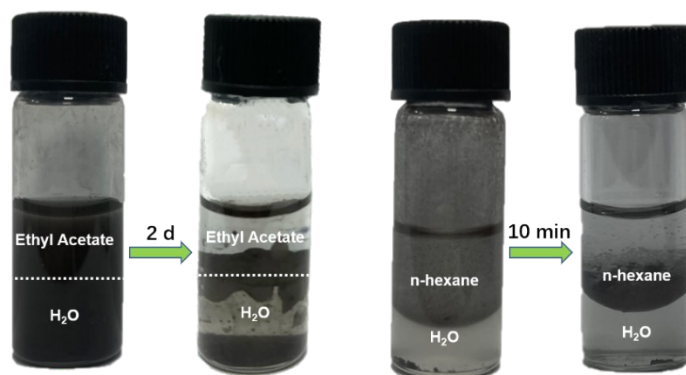
Fig. S7 The wettability of Cu@Co@GC/NC in a biphasic solution ( V_{H_2O}/V_{oil} = 1:1 ) before and after 2 days, the organic upper layer (ethyl acetate or n-hexane) and aqueous bottom layer (water).
