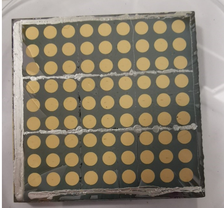
Figure S2. 81 individual Sb 2 Se 3 PV devices on a 5x5 cm 2 FTO glass.
