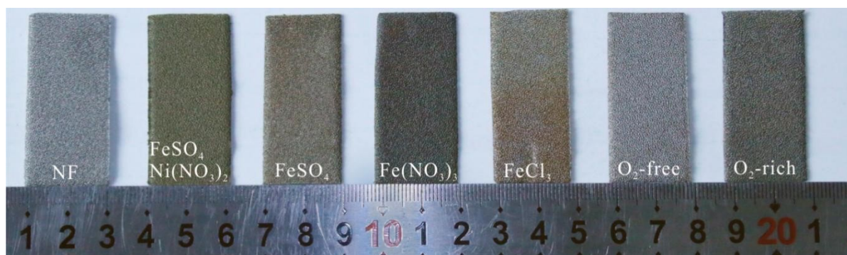
Fig. S3. The digital photographs of bare NF and NF treated by immersion in \text{FeSO}_4/\text{Ni}(\text{NO}_3)_2 , \text{FeSO}_4 , \text{Fe}(\text{NO}_3)_3 , \text{FeCl}_3 , \text{O}_2 -free and \text{O}_2 -rich \text{FeSO}_4/\text{Ni}(\text{NO}_3)_2 solution.
