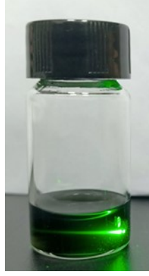
Figure S1 Stable MXene colloidal with Tyndall effect
