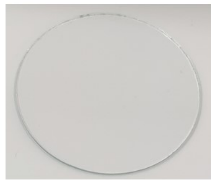
(b) Single \text{LiNbO}_3 film
