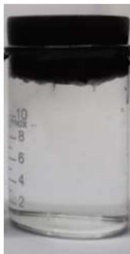
**Figure S11.** Digital photo of TSAS-3 after 14 days immersion.
