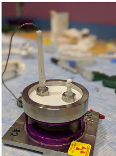
Figure S1 A picture of the cell used for neutron reflectivity experiments.
