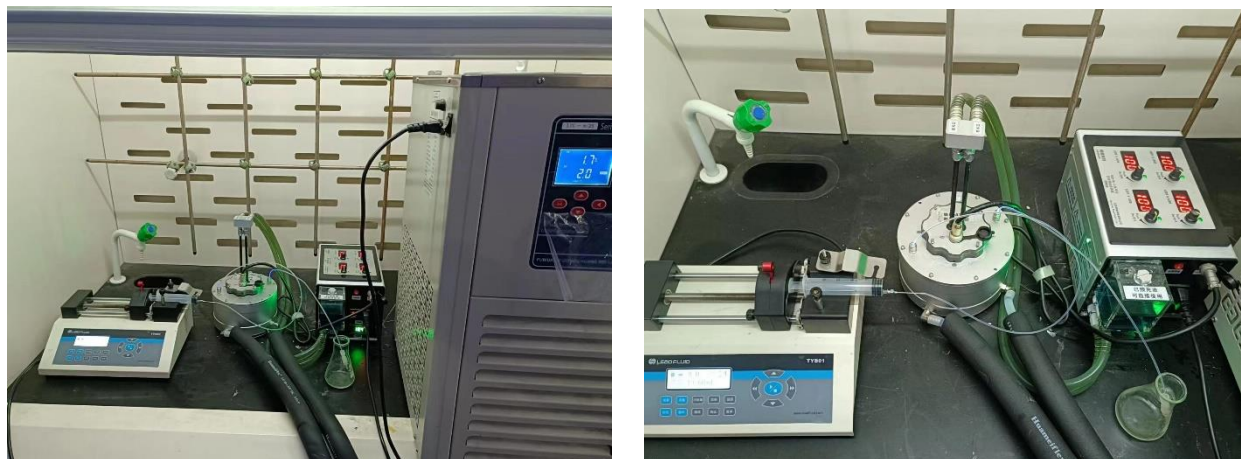
Figure S3. Picture of the Flow Photoreactor
