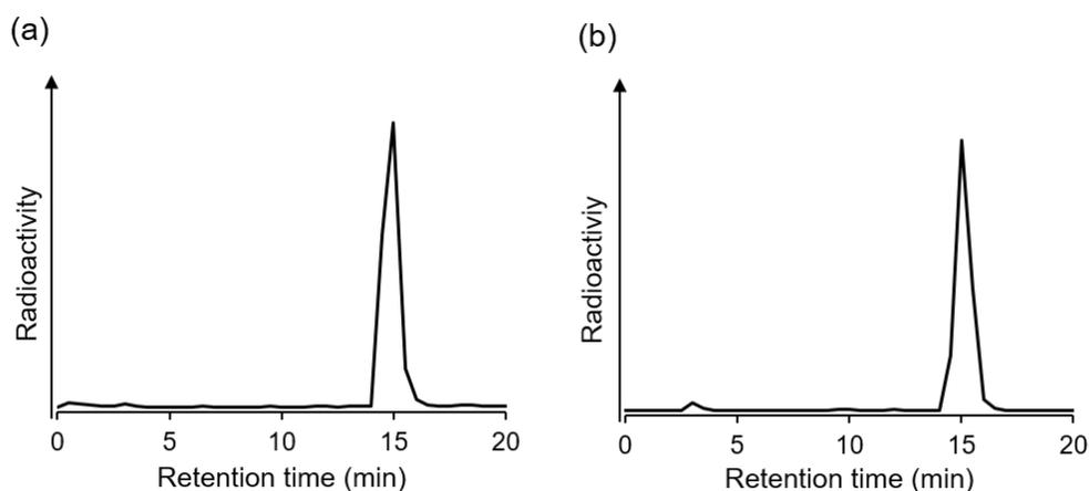
**Figure S8.** (a) HPLC chromatogram of [ $^{125}\text{I}$ ]4 before the incubation in murine plasma.
