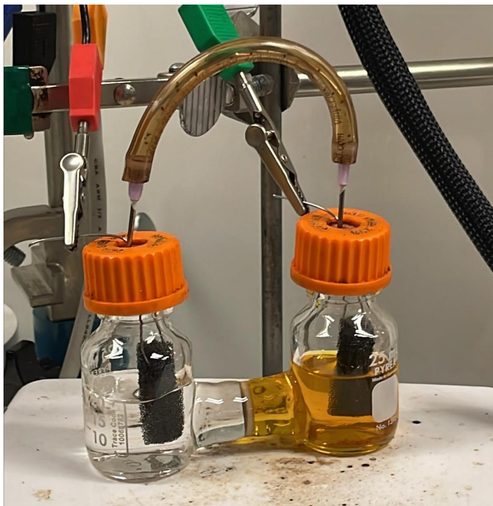
Figure S1: Picture of electrochemical setup in an H-Cell performed with a Tygon tube used to balance pressure. Reticulated Vitreous Carbon electrodes were employed as cathode and anode and connected to the potentiostat via stainless steel wires that are kept out of solution.
