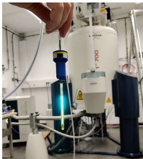
Figure S24. NMR sample with quartz glass insert and optical fibre for in-situ illumination during NMR experiments.
