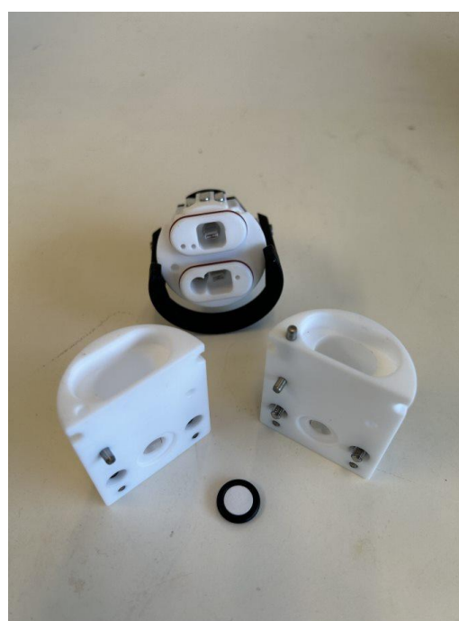
Figure S5 , IKA ElectraSyn 2.0 and an ElectraSyn Pro-divide fitted with a glass frit (pore size 10-16 \mu\text{m} ) and ElectraSyn glassy carbon electrodes (4 x 0.8 x 0.2 cm).
