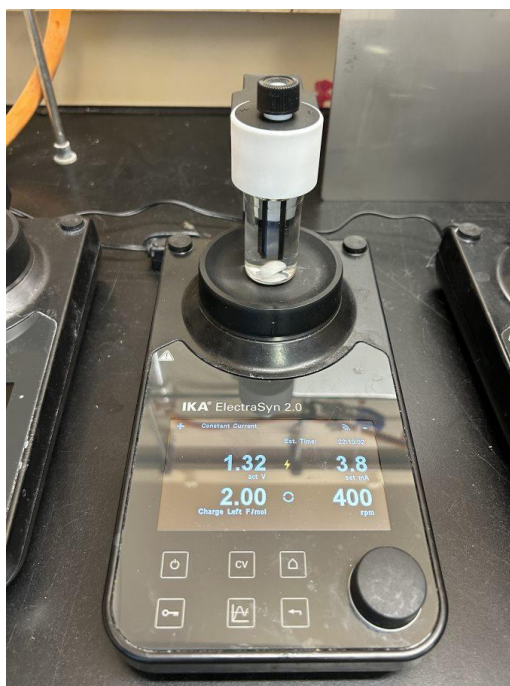
Figure S8 , IKA ElectraSyn 2.0 and a 20 mL ElectraSyn undivided vial fitted with ElectraSyn glassy carbon electrodes (4 x 0.8 x 0.2 cm; 6.1 cm 2 area exposed to the electrolyte).
