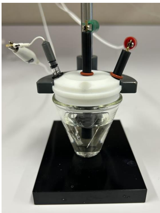
Figure S3 , Three-electrode cell made up of a BASi Ag/AgCl (3 M NaCl) reference electrode, a BASi glassy carbon working electrode ( \varnothing 3.0 mm) and a BASi platinum wire auxiliary electrode (7.5 cm).
