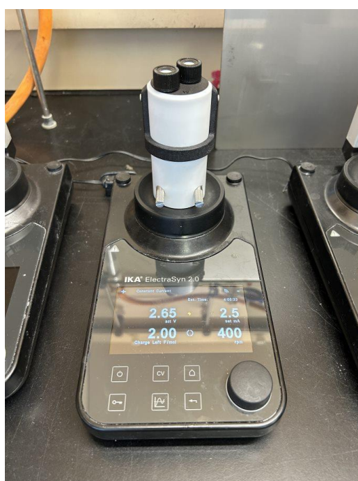
Figure S5 , IKA ElectraSyn 2.0 and an ElectraSyn Pro-divide fitted with a glass frit (pore size 10-16 \mu\text{m} ) and ElectraSyn glassy carbon electrodes (4 x 0.8 x 0.2 cm).
