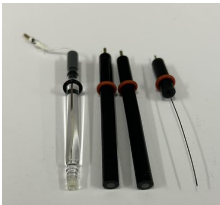
Figure S2 , Electrodes used for cyclic voltammetry; from left to right, BASi Ag/AgCl (3 M NaCl) reference electrode, 2 x BASi glassy carbon electrodes ( \varnothing 3.0 mm) and a BASi platinum wire auxiliary electrode (7.5 cm).
