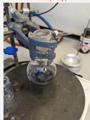
Fig S3: NiCl 2 ·6H 2 O (5 mol%) + NaBH 4 (4 eq.) + butenolide (1 eq.) in MeOH
