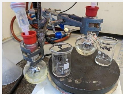
Fig S2: NiCl 2 ·6H 2 O (5 mol%) + NaBH 4 (4 eq.) + butenolide (1 eq.) in THF or PhMe
