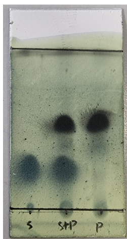
Figure 1: TLC (10% EtOAc/hexane) of reaction between cyclohexenone 23 and silyl enol ether 22 , t = 1.5 hours.
