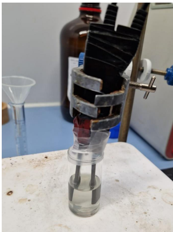
Figure S1. Undivided electrochemical cell with graphite electrodes
