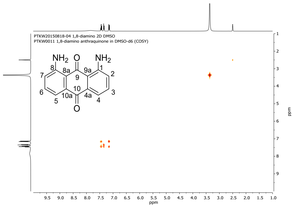
SI 4 COSY ^1\text{H} - ^1\text{H} spectrum of 1,8-diaminoanthraquinone ( 4 ) in DMSO- d_6 (400 MHz)
