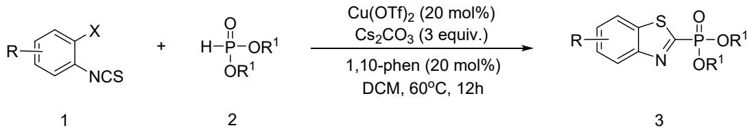
In a schlenk sealed tube equipped with a stirrer, **1** (0.20 mmol, 1.0 equiv.) and **2** (0.4mmol, 2.0 equiv.), Cu(OTf)<sub>2</sub> (20 mol%), 1,10-phen (20 mol%), CsCO<sub>3</sub> (0.6 mmol, 3 equiv.) and DCM (2mL) were added. Place the sealed tube in an oil bath which is preheated to 60 °C. The mixture was stirred for 12h. Then, the mixture was concentrated in vacuo, and purified by column chromatography on silica gels (ethyl acetate/petroleum ether, 4:5) to get **3**.
