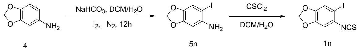
In a 150 mL round bottom flask equipped with a magnetic stirring bar, **4**(685mg, 5.0mmol) and  $\text{NaHCO}_3$  (1.26g, 15.0mmol) was added. Then,  $\text{DCM}/\text{H}_2\text{O}$  (33mL, 2:1)
