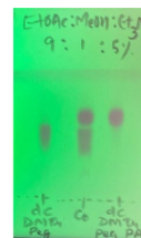
TLC (SiO 2 ) for compound 1a . Left lane: compound 14 ; middle lane: co-spot of compounds on left and right lanes; right lane: compound 1a (diastereomers). Eluent: EtOAc/MeOH 9:1 with 5% Et 3 N.
