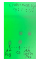
TLC (SiO 2 ) for compound 20 . Left lane: compound 19 ; middle lane: co-spot of compounds on left and right lanes; right lane: compound 20 . Eluent: EtOAc/MeOH 9:1 with 5% EtN.
