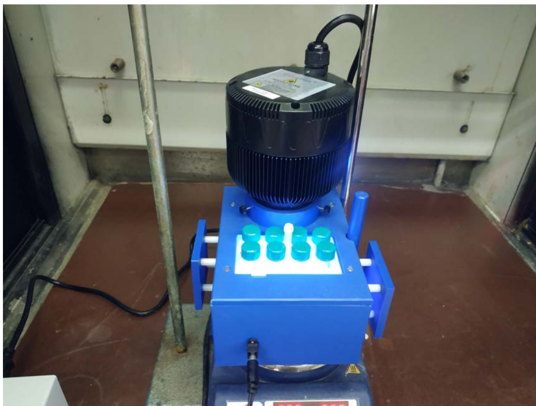
Figure S1. Photochemical set-up. Solvent screening.
