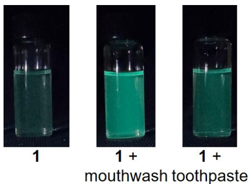
Figure S42. Photograph of solutions of compound 1 without analyte, and in the presence of mouthwash and toothpaste, taken under 365 nm excitation ( [1] = 4 \mu\text{M} in acetonitrile)
