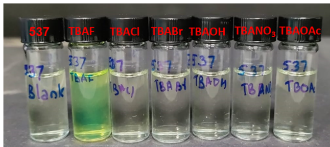
Figure S62. Images taken under ambient light of solutions of compound 1 , followed by exposure to no analyte (left-most vial), or exposure to analytes: TBAF, TBACl, TBABr, TBAOH, TBANO 3 , or TBAOAc ([ 1 ] = 10 μM; [analyte] = 10 μM)
