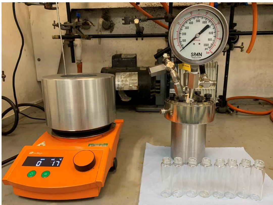
Figure 1 - Hydrogenation reaction setup
