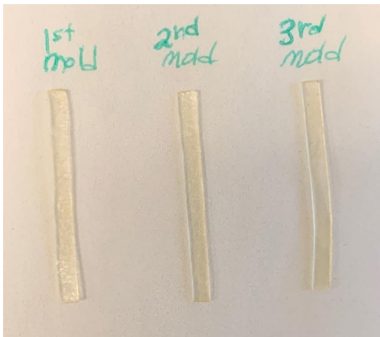
Figure S17. Images of molded PHMA networks synthesized with 5 mol% BiTEBES methacrylate and 1 mol% AIBN.
