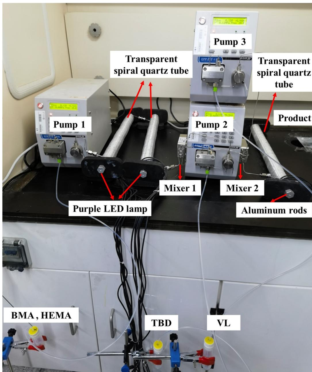
**Fig. S5** Photograph of continuous flow setup for preparation of grafted polyesters through successive photocontrolled BIT-RDRP and ROP strategy at room temperature. The temperature was controlled by mechanical ventilation and monitored by thermal imager.
