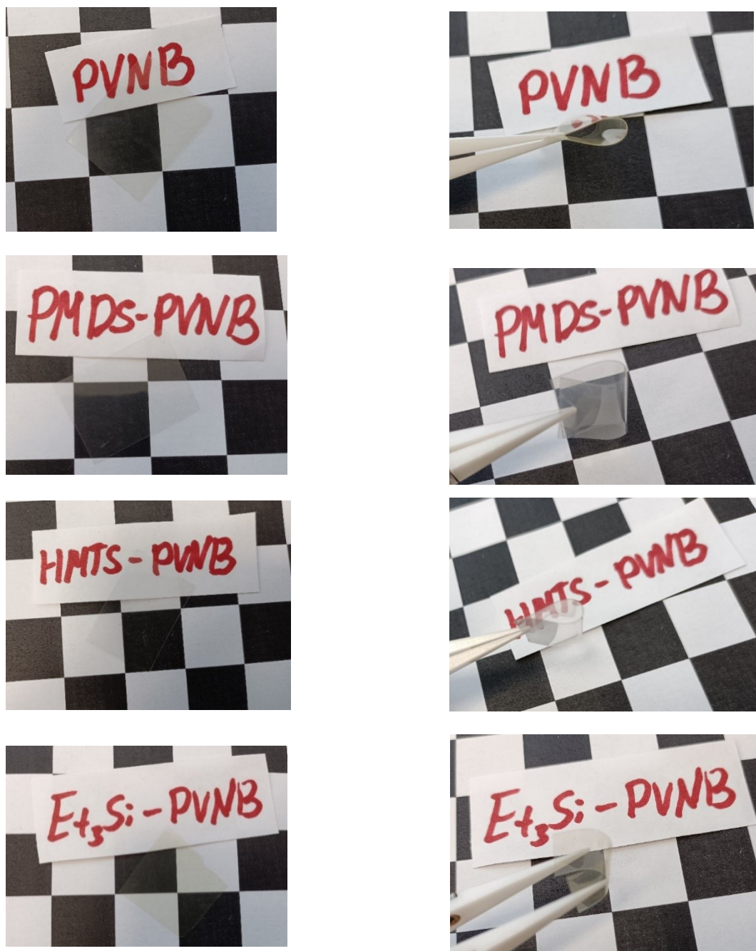
Fig. S23 Photos of thin films based on PVNB and modified silicon-containing polymers obtained from PVNB.
