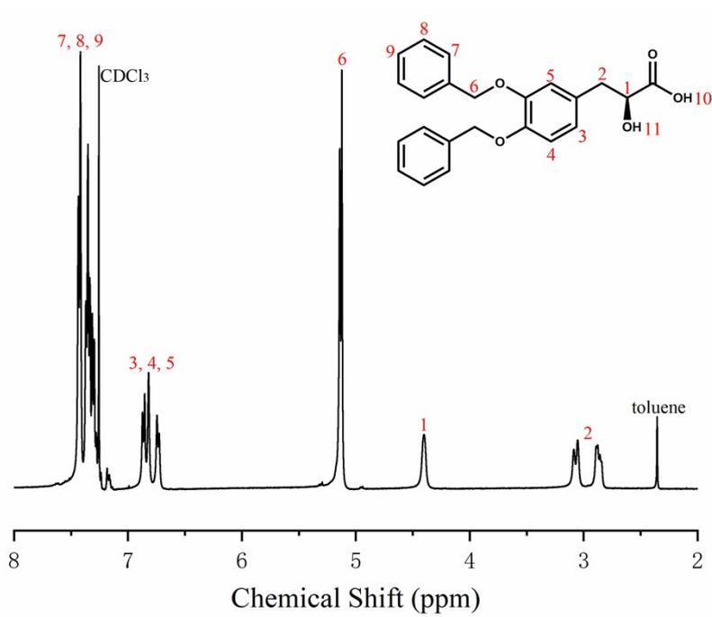
**Fig. S4**  $^1\text{H}$  NMR spectrum of D4 in  $\text{CDCl}_3$ .
