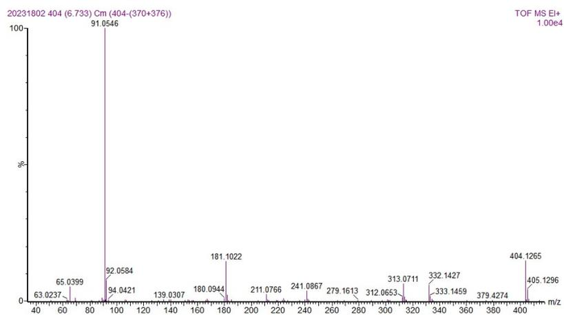
**Fig. S6** Electron-impact-ionization mass spectrum of *L*-Dopa(Bn)OCA.
