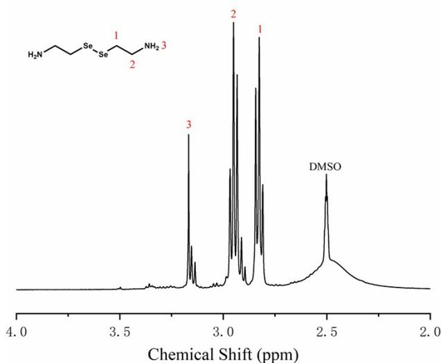
Fig. S10  $^1\text{H}$  NMR spectrum of selenocystamine in  $\text{DMSO-d}_6$ .
