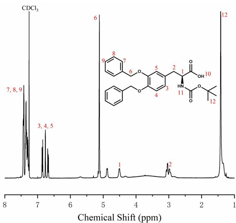
Fig. S2 <sup>1</sup>H NMR spectrum of D2 in CDCl<sub>3</sub>.
