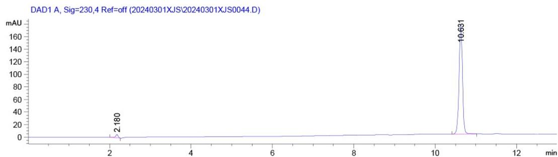
**Fig. S8** Ultra-high performance liquid chromatogram of (+)- $\alpha$ -methylbenzylamine adduct of Dopa(Bn)OCA.
