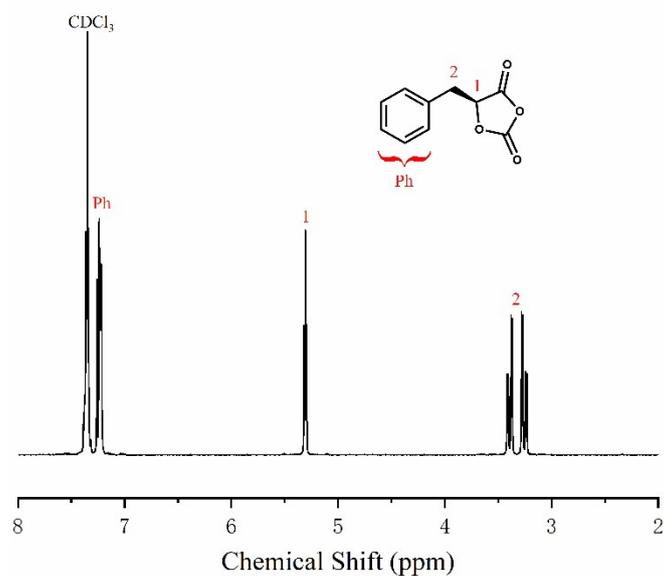
Fig. S9  $^1\text{H}$  NMR spectrum of  $L$ -PheOCA in  $\text{CDCl}_3$ .
