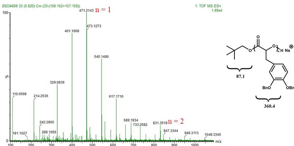
Fig. S12 Electrospray-ionization mass spectrum (Region  $m/z$  100 to 1200) of polyester prepared by polymerization of  $L$ -Dopa(Bn)OCA with *neo*-pentanol (Toluene,  $25^\circ\text{C}$ ,  $[\text{OCA}]_0/[\text{ROH}]_0/[\text{MOP}]_0 = 5/1/1$ ).
