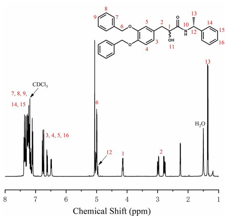
**Fig. S7**  $^1\text{H}$  NMR spectrum of (+)- $\alpha$ -methylbenzylamine adduct of Dopa(Bn)OCA in  $\text{CDCl}_3$ .
