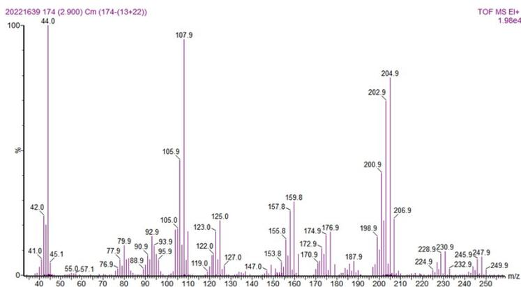
Fig. S11 Electron-impact-ionization mass spectrum of selenocystamine.
