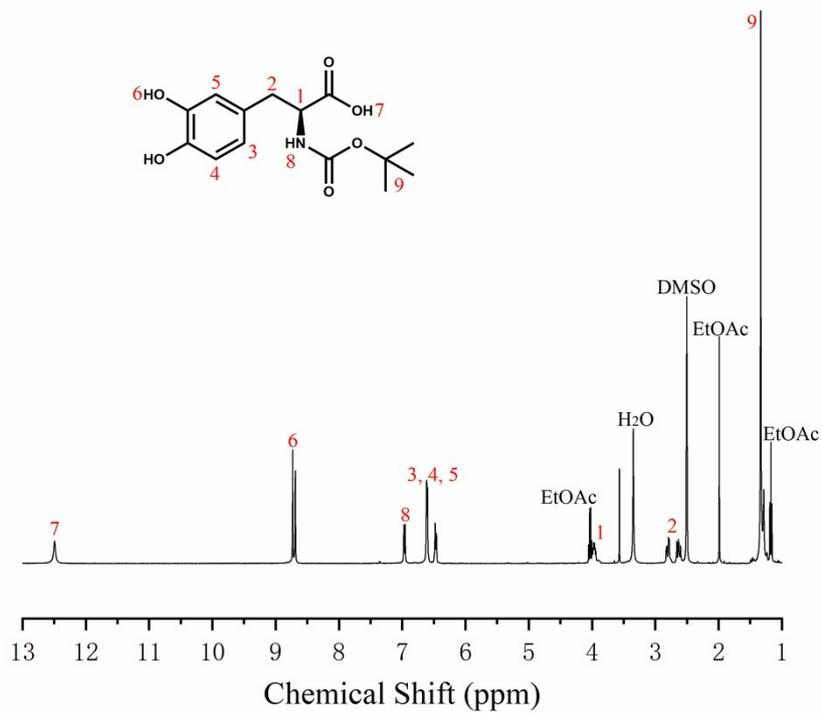
Fig. S1 <sup>1</sup>H NMR spectrum of D1 in DMSO-d<sub>6</sub>.
