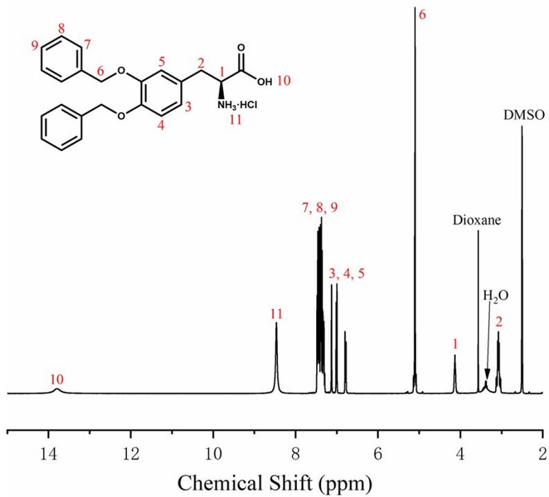
**Fig. S3**  $^1\text{H}$  NMR spectrum of D3 in  $\text{DMSO-d}_6$ .
