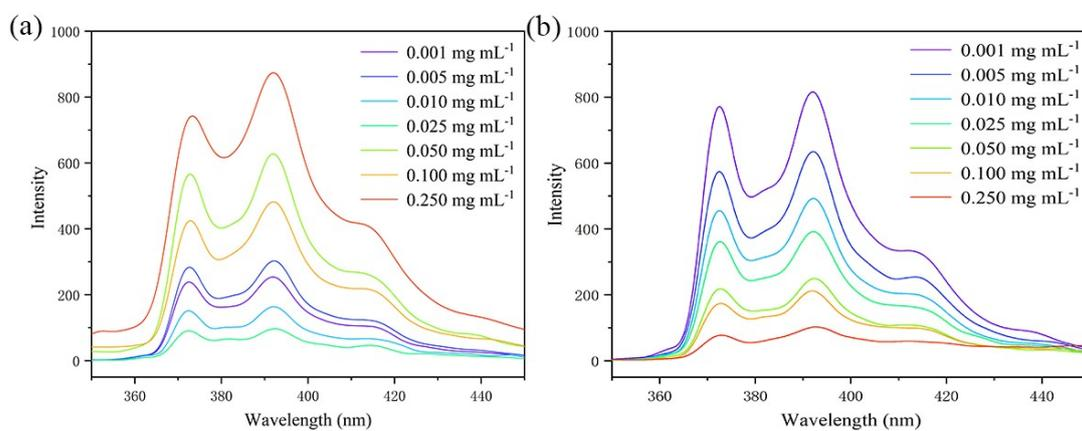
**Fig. S15** The emission spectra of pyrene in mPEG<sub>5k</sub>-*b*-poly(DopaOCA)<sub>20</sub> solution (a) before and (b) after cross-linking at different concentrations ( $\lambda_{\text{ex}} = 334 \text{ nm}$ ).
