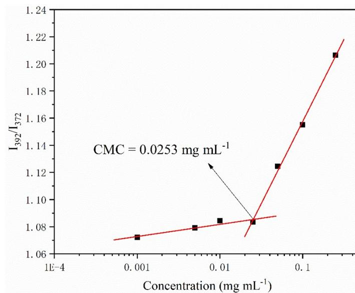
**Fig. S16** The intensity ratio ( $I_{392}/I_{372}$ ) as a function of the concentration of mPEG<sub>5k</sub>-*b*-poly(DopaOCA)<sub>20</sub> solution.
