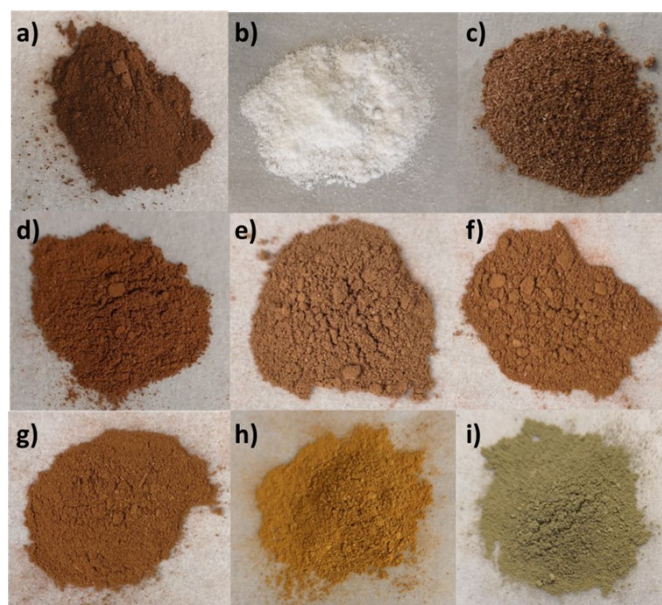
Figure S3. Images of starting materials and neat BM products. a) \text{Co(NCS)}_2 (1 mmol), b) 4,4'-bipyridine (2 mmol), c) manual mixture of \text{Co(NCS)}_2 (1 mmol) and 4,4'-bipyridine (2 mmol); neat BM (25 Hz) of \text{Co(NCS)}_2 (1 mmol) and 4,4'-bipyridine (2 mmol) for d) 5 min, e) 10 min, f) 15 min, g) 30 min, h) 1 h, and i) 2 h.
