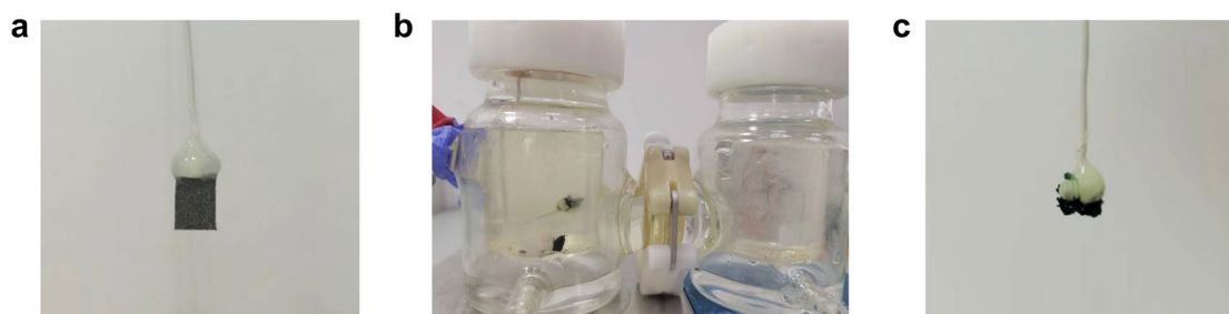
Fig. S8. Photographs of NiCoFe-Bi/NF electrode: (a) as-prepared; (b, c) after stability test at 500 \text{ mA cm}^{-2} for 15 h in artificial seawater at pH 14 with 0.05 mM Fe(II) ions.
