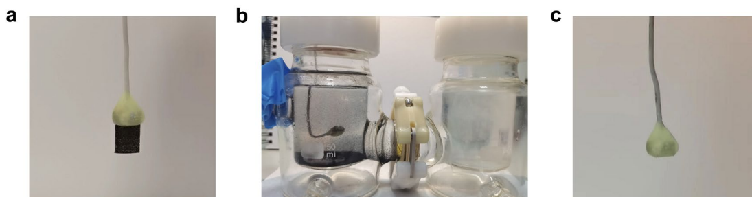
Fig. S5. Photographs of NiCoFe-Bi/NF electrode: (a) as-prepared; (b, c) after stability test at 100 \text{ mA cm}^{-2} for 20 min in artificial seawater at pH 7.65.
