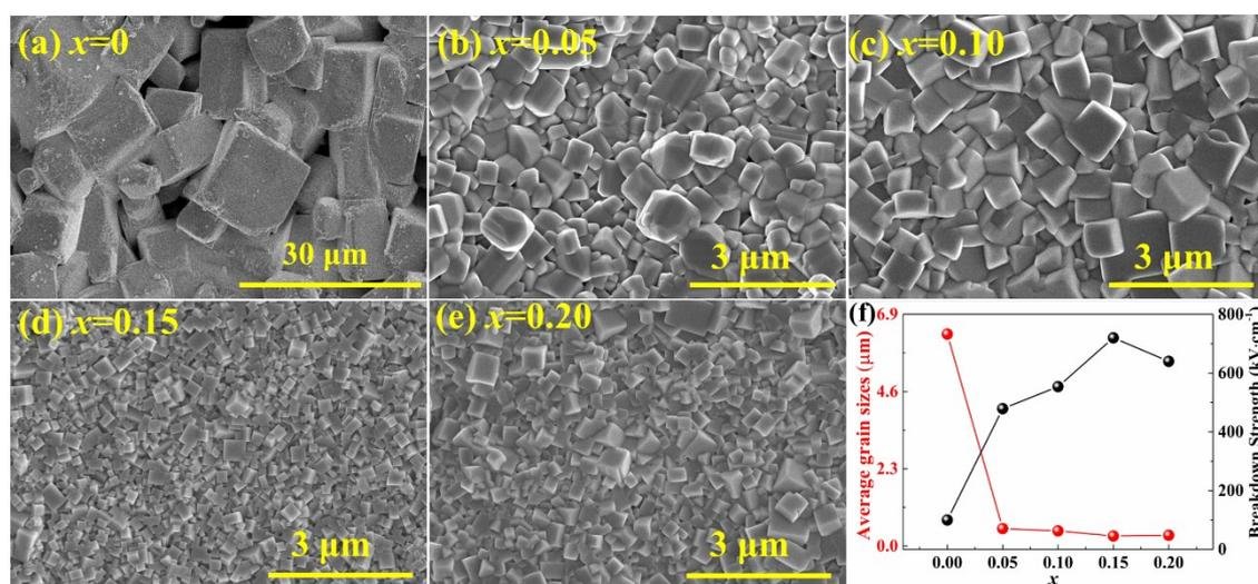
**Fig. S1** SEM images of the (1-x)KNN-xBMT ceramics: (a)  $x=0$ ; (b)  $x=0.05$ ; (c)  $x=0.10$ ; (d)  $x=0.15$ ; (e)  $x=0.20$ ; (f) Average grain sizes and BDS of (1-x)KNN-xBMT ceramics.
