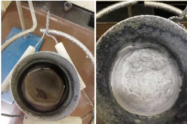
Figure S6: Molten mixture over a gas flame of potassium hydroxide and niobium pentoxide for synthesizing KNb. A nickel crucible is used (left). Cooled melt of KNb and potassium hydroxide after KNb synthesis. A nickel crucible is used (right).
