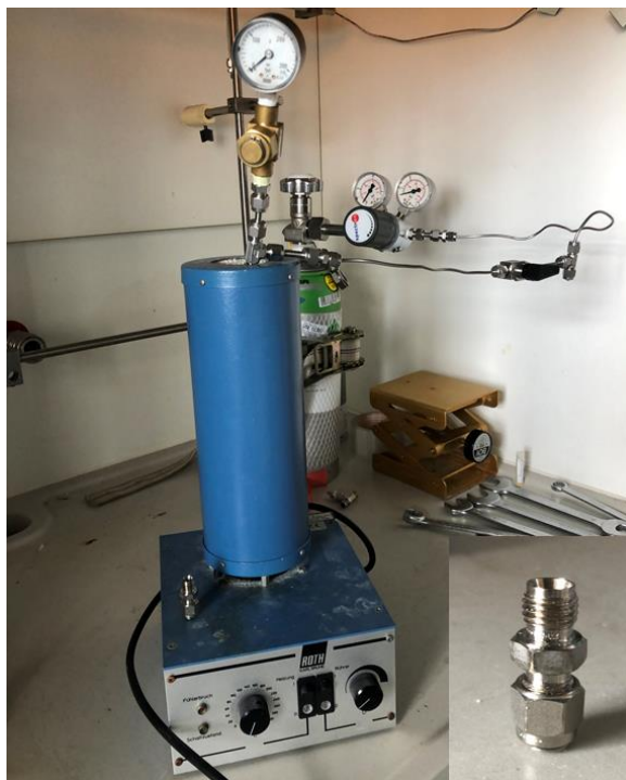
Figure S6. Home-built apparatus for gas loading with a sample chamber shown in the inset.
