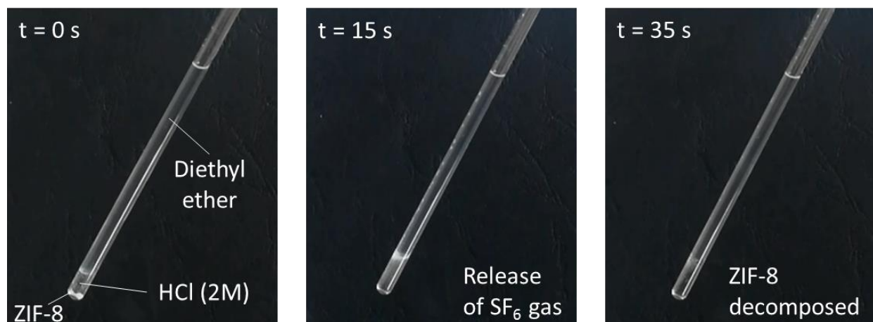
Figure S33. Photographs of an acid-induced gas release from ZIF-8(s) loaded with \text{SF}_6 (Sample 1a2). A sample of ZIF-8(s) (ca. 5 mg) was exposed to a 2M aqueous solution of HCl (ca. 0.15 mL). To improve the visualization of the gas release, the sample was layered with diethyl ether (ca. 0.9 mL) before the acid was added; however, the layering is not necessary and does not affect the result of the experiment. A video capturing the experiment as well as a control experiment without the loaded gas guest is available as Electronic Supplementary File.
