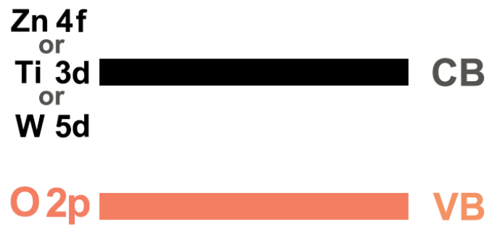
Fig. S19 Schematic diagram of the band structure of ZnO, TiO 2 , and WO 3 .
