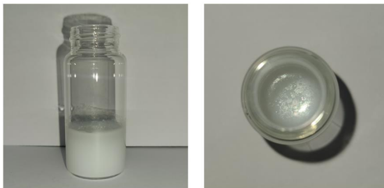
Fig. S4 Photographs of as-synthesised ZIF-8 crystal solution with 0.10% xylene-based microemulsion right after the synthesis was terminated. For better visual aid, a scale-up reaction was performed (total volume: 6 mL).
