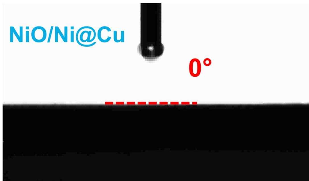
Figure S15. Contact angle measurement of NiO/Ni@Cu.
